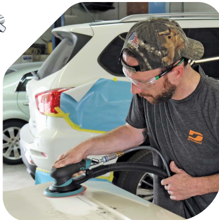
3/16" (5 mm) DIA. ORBIT General Sanding
