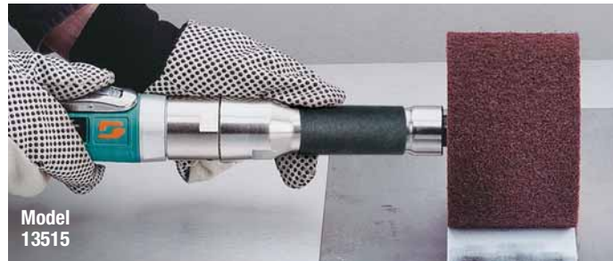
13515 Dynastraight® sets grain pattern in stainless steel.
