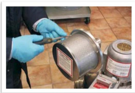
Remove the 3 screws on the HEPA/ULPA housing using a Philips Screw Driver.
