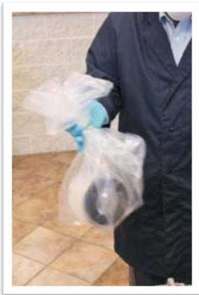
**The HEPA/ULPA filter is now sealed inside of the poly liner and can be disposed of according to local governmental laws. (*Conductive poly liners are available.*)**
