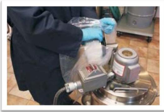
**Place a poly liner around the now exposed HEPA/ULPA filter. Carefully remove the HEPA/ULPA filter from the back plate. Gently place the HEPA/ULPA filter into the poly liner. Gently twist the poly liner and then seal it with a tie wrap.**
