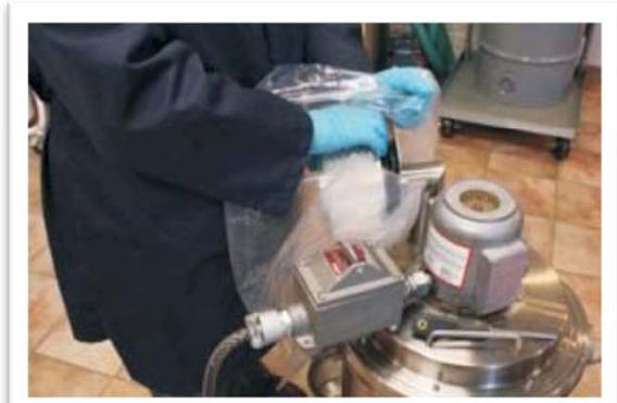
Place a poly liner around the now exposed HEPA/ULPA filter. Carefully remove the HEPA/ULPA filter from the back plate. Gently place the HEPA/ULPA filter into the poly liner. Gently twist the poly liner and then seal it with a tie wrap.
