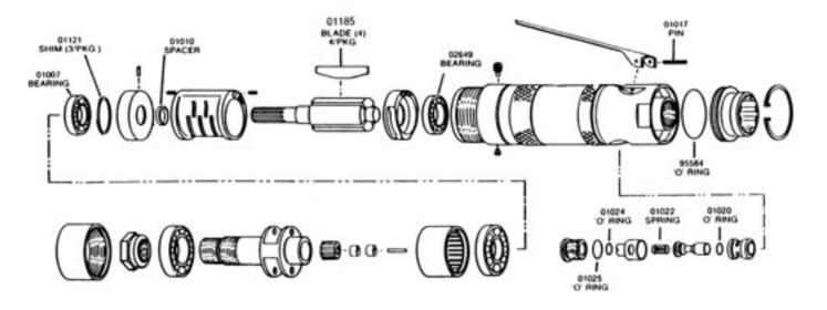
NOTE: WHEN REASSEMBLING MOTORS ADD A DROP OF LOCTITE®
