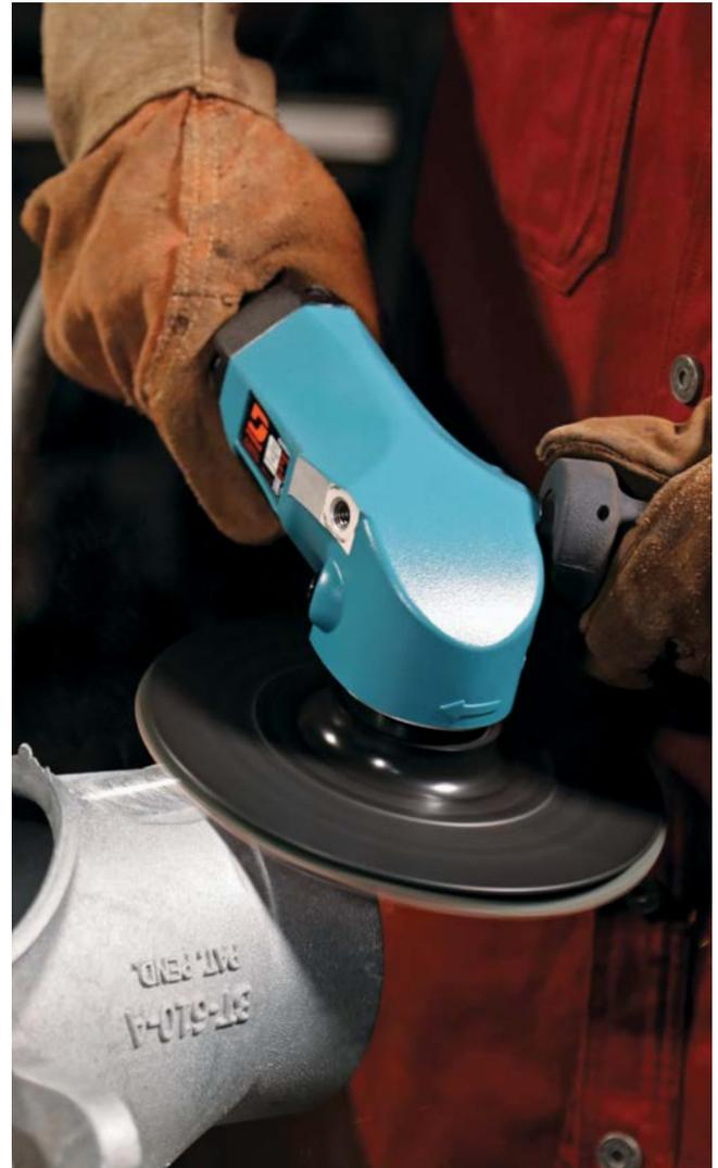
**TECH TIP** Always present the tool and abrasive to the work piece at a 10° – 15° angle for efficient abrasive use and to prevent gouging.
