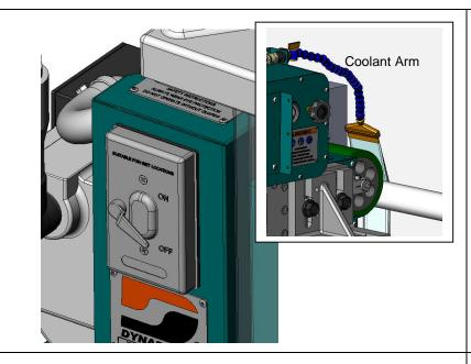
Be sure that your tool coolant arm is pointing toward the proper location for lathe bed collection.
