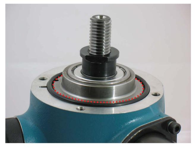
14. Install 95881 O-Ring against front bearing plate.
