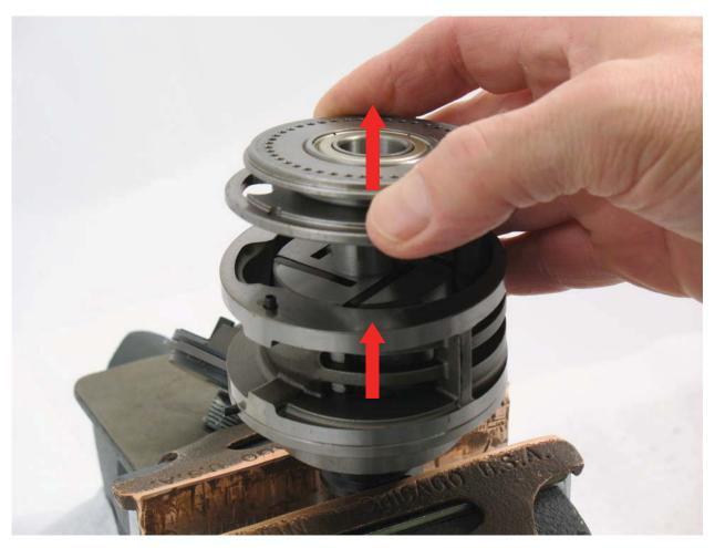
4. Remove 55202 Rear Bearing Plate, bearing, cylinder, and vanes.
