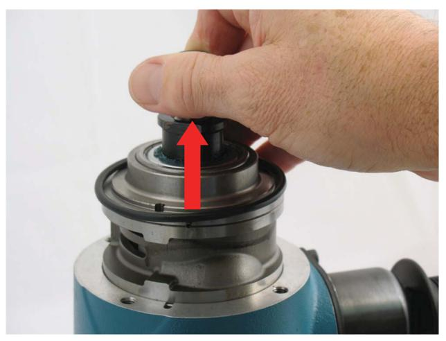
2. Remove 95881 O-Ring and motor from housing.
