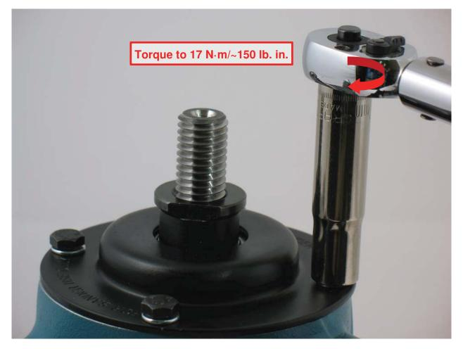
15. Install housing cover or guard. Fasten with 50508 Screws and 95757 Washers. Torque to 17 N·m/ $\sim$ 150 lb. in.
