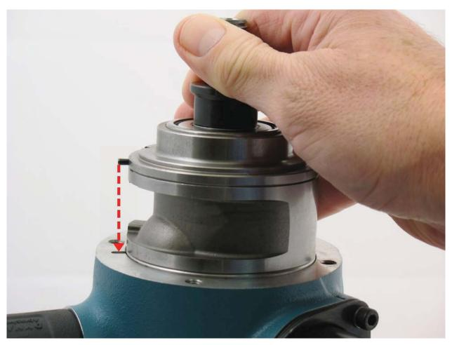
**13.** Carefully install motor in housing.
