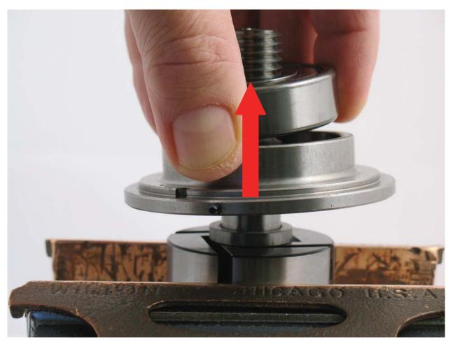
6. Remove front bearing plate, bearing, shims and 55223 Spacer from rotor.
