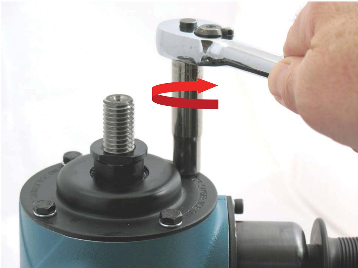
1. Use 10 mm socket wrench to remove **50508** Screws.
