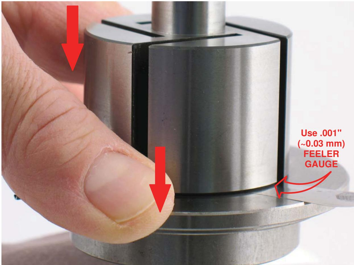
4. Place end rotor spindle on a flat surface. Push down on bearing plate, and use a .001" (~0.03 mm) thick feeler gauge to check clearance between front bearing plate and rotor.
