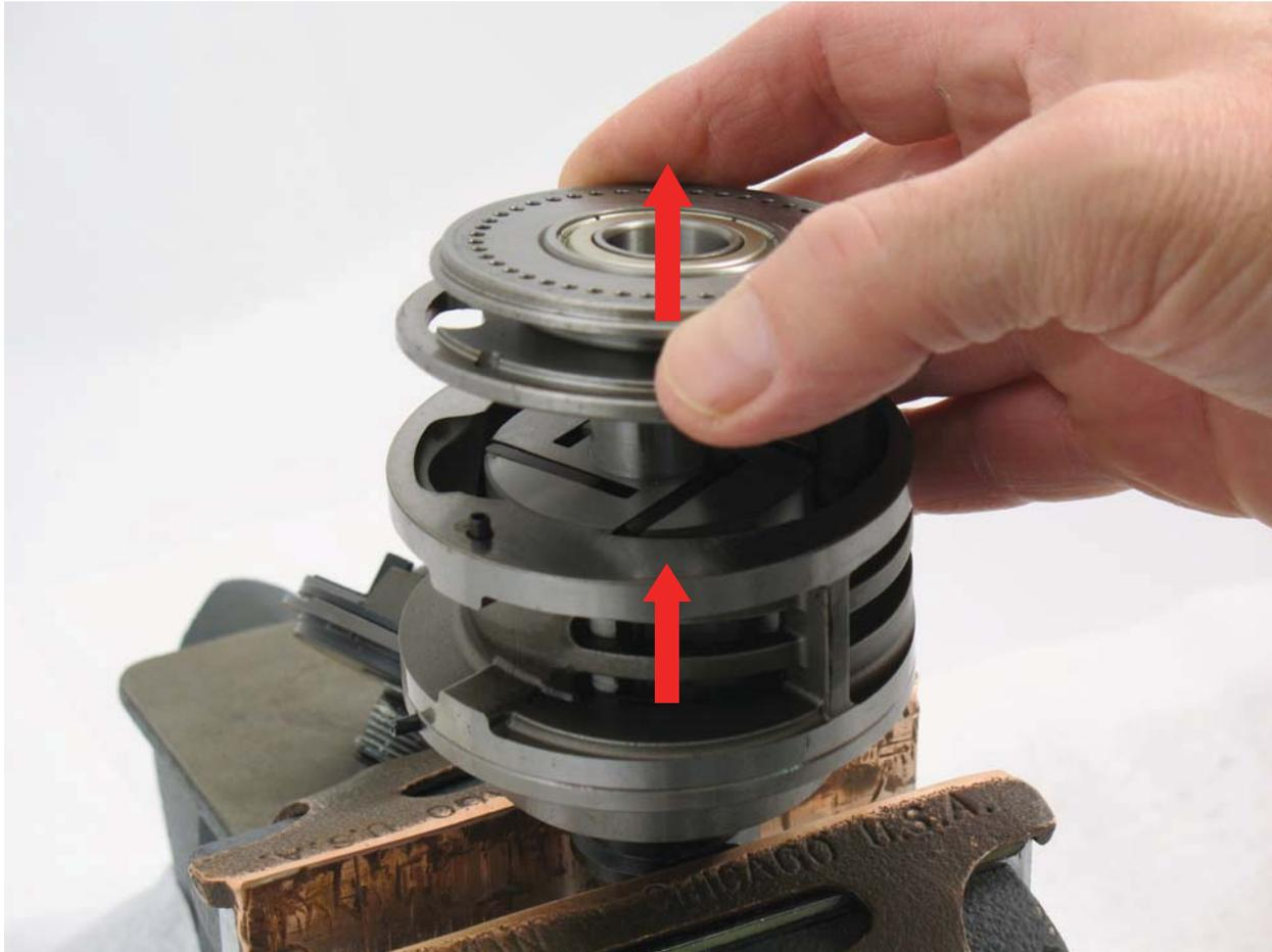
4. Remove **55202** Rear Bearing Plate, bearing, cylinder, and vanes.
