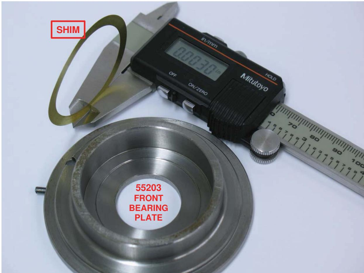
2. Install **52470** Shim (.003" or ~0.08 mm, thick).
