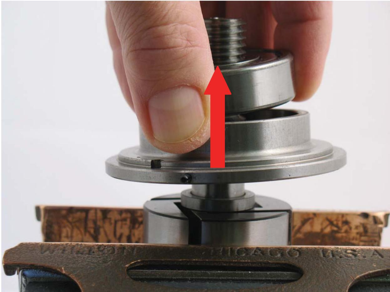
6. Remove front bearing plate, bearing, shims and **55223** Spacer from rotor.
