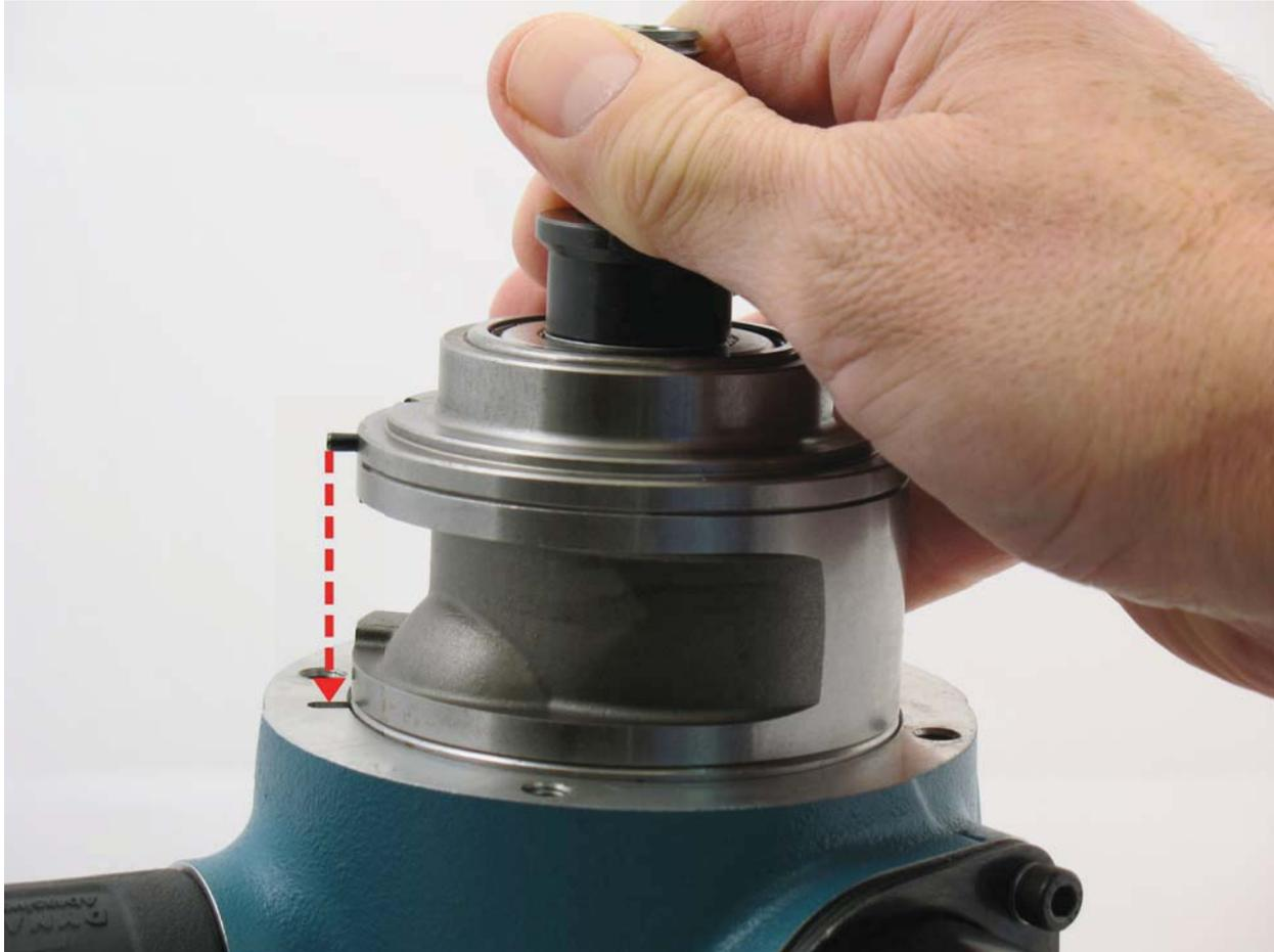
13. Carefully install motor in housing.
