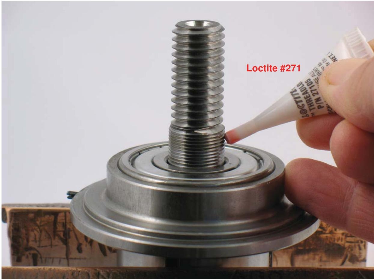
5. Fasten rotor in vise with spindle pointing up.
