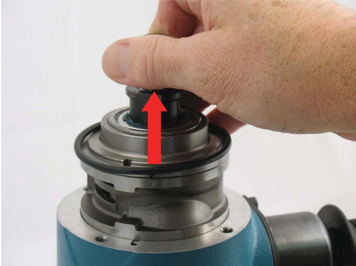
2. Remove **95881** O-Ring and motor from housing.
