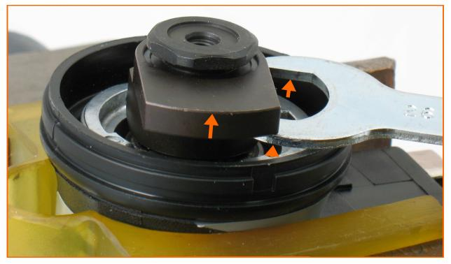
4. Pry-up, under the motor shaft balancer to remove the air motor from the housing.
