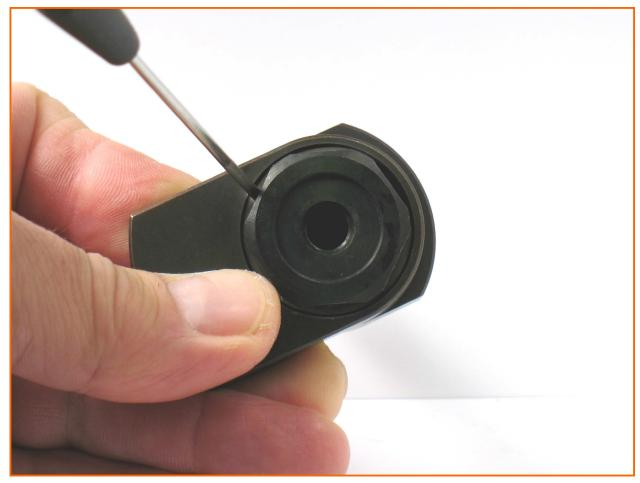
3. Compress the **95630** Snap Ring into the groove in the motor shaft balancer.
