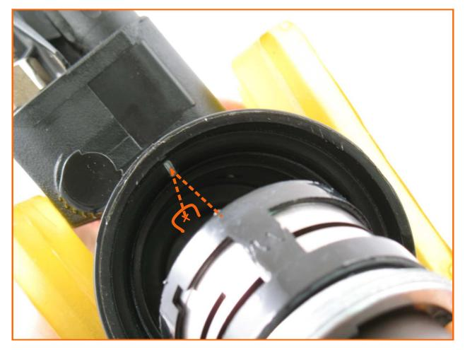
**14.** Sight the cylinder line-up pin with the notch on the inside of the housing. Also, sight the line-up guide on the housing and install the motor.
