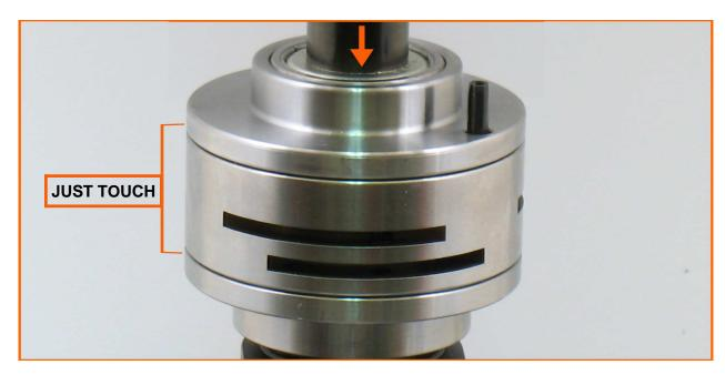
10. Use the small diameter end of the 57091 Bearing Press Tool and the arbor press to install the bearing/plate onto the motor shaft balancer. Notice: Carefully press the bearing and plate down until it <u>just touches the cylinder</u>. This will establish a close fit between the bearing plates and the cylinder.
