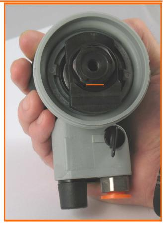
**18.** Align the balancer shaft with matching hex socket and install.
