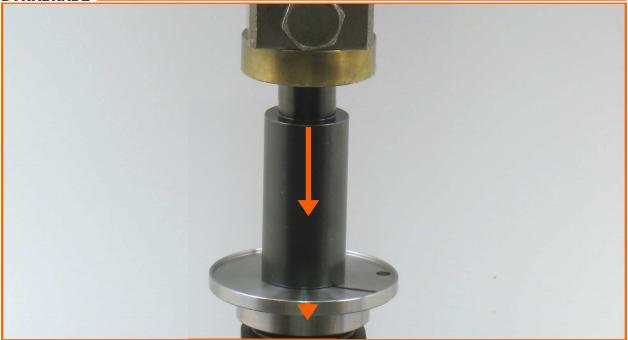
**5.** Use the large diameter end of the **57091** Bearing Press Tool, and the arbor press to install the **57057** Front Bearing Plate.
