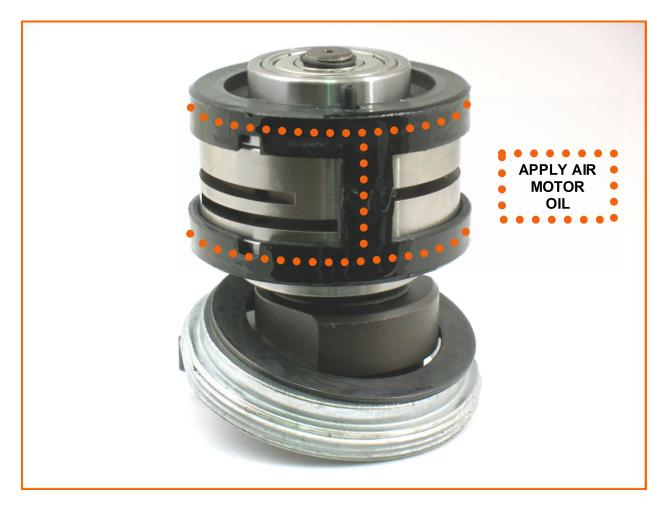
13. Apply air motor oil to the rubber rings.
