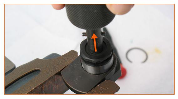
Use the 56056 Bearing Puller to remove the balancer shaft and the 56052 Bearing.
