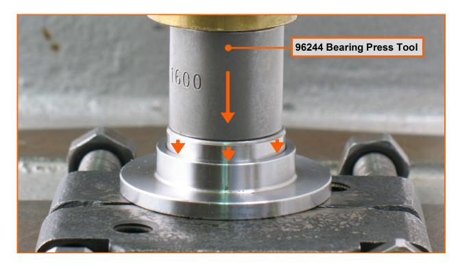
**8.** If necessary, use the **RAISED OUTSIDE DIAMETER** of the **96244** Bearing Press Tool and the arbor press to install the **01206** Bearing into the **57056** Rear Bearing Plate.
