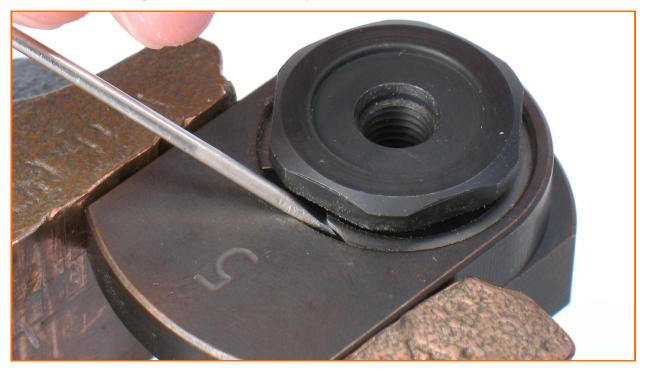
a) Fasten the counterweight in a vise with aluminum or bronze jaws so that the hex of the 57069 Balancer Shaft is pointing up. Use a thin slot-blade screwdriver to pick-out the end of the 95630 Snap Ring and remove the snap ring from the motor shaft balancer.
