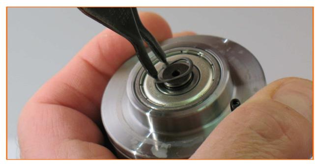
5. Use retaining ring pliers to remove the 95626 Retaining Ring.
