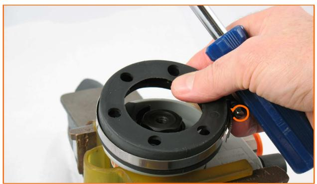
2. Use a slot-blade screwdriver to loosen the **96116** Clamp. Remove the clamp, **57822** Boot and **57823** Pad Mount.
