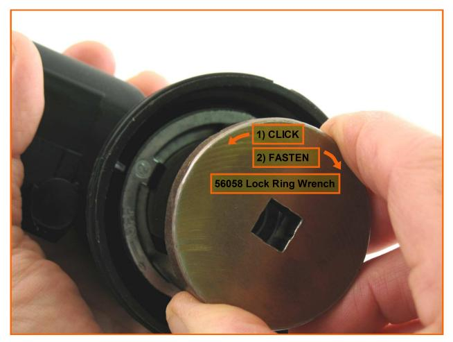
15. By hand, use the 56058 Lock Ring Wrench to locate thread and fasten motor in housing.
