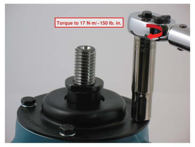
15. Install housing cover or guard. Fasten with 50508 Screws and 95757 Washers. Torque to 17 N $\cdot$ m/~150 lb. in.
