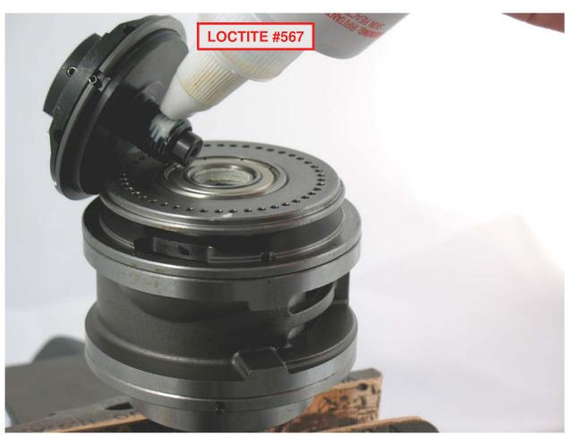
10. Apply a small amount of Loctite #567, or equivalent to threads of governor.
