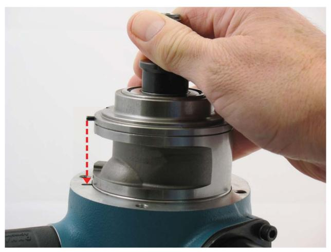
**13.** Carefully install motor in housing.
