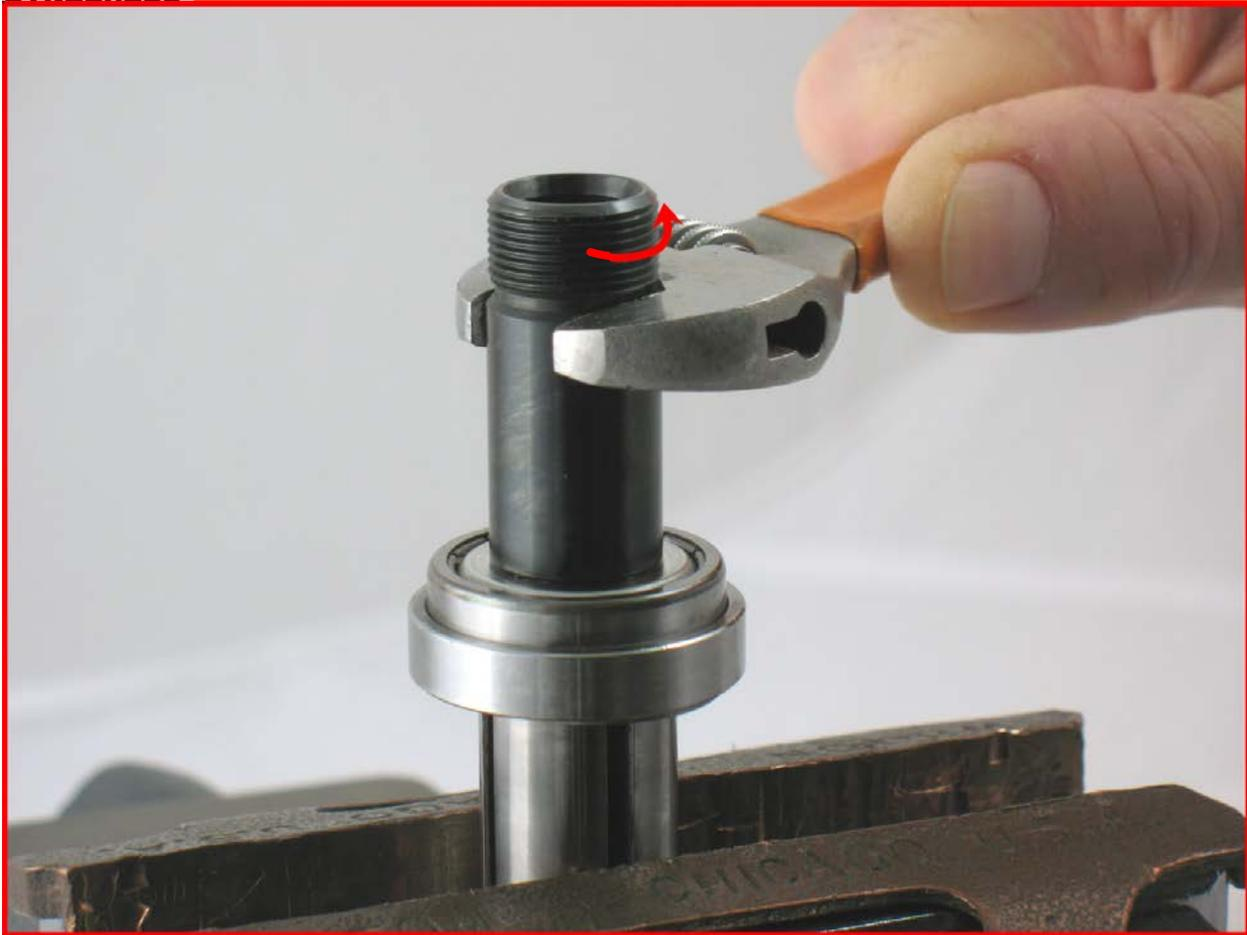
6. Fasten the rotor in the vise with aluminum or bronze jaws so that the work spindle is pointing up. Use an adjustable wrench to remove the collet body. Turn counterclockwise.
