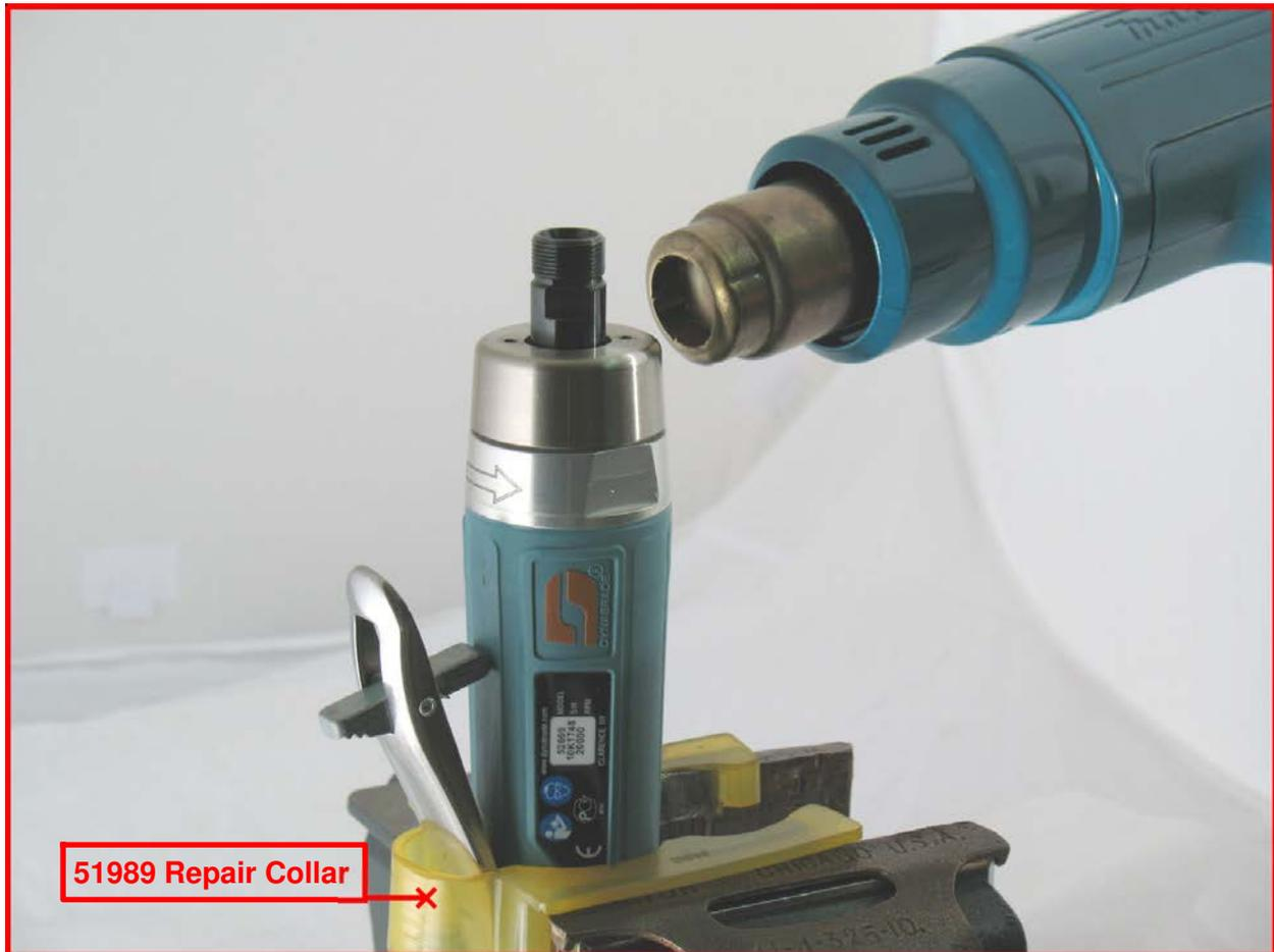
1. Position the **51989** Repair Collar around the motor housing. Fasten the tool in a vise so that the work spindle is pointing up. Use a HEAT GUN to warm the Housing Cover: **51947**, **51962**, **51972** and soften the thread adhesive.
