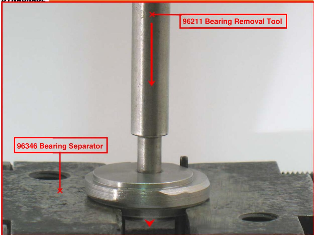
5. Use the **96346** Bearing Separator (2"), the arbor press and the **96211** Bearing Removal Tool to remove the **02057** Bearing from the rear bearing plate.
