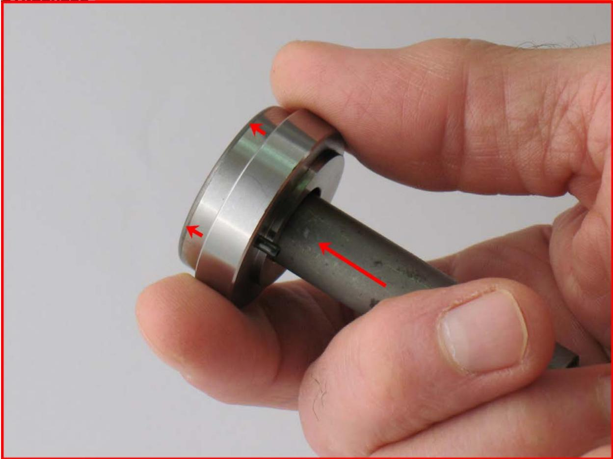
7. By hand, use a press tool to remove the **54520** Bearing from the front bearing plate.
