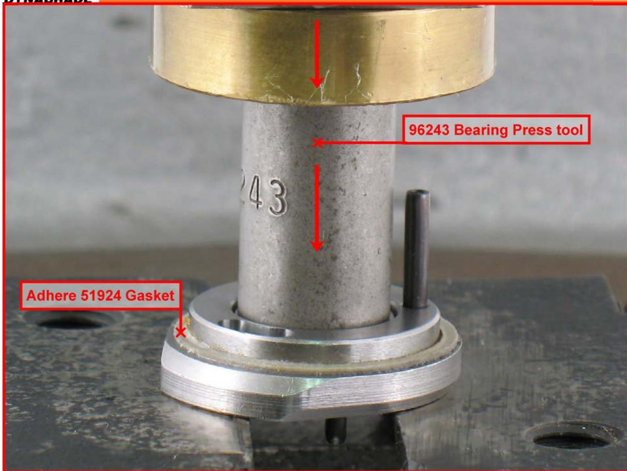
4. Use solvent to remove all oil from **51923** Rear Bearing Plate. Peel backing from **51924** Gasket and adhere adhesive side to the bearing plate.
