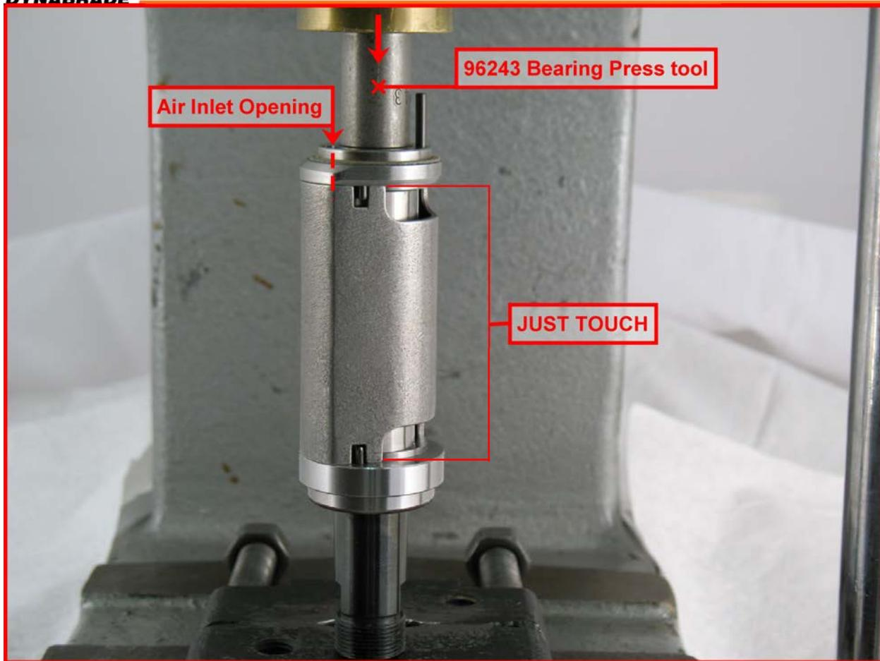
6. Install the **51925** Cylinder so that the air inlet opening in the **51923** Rear Bearing Plate will line-up with the air inlet in the cylinder.
