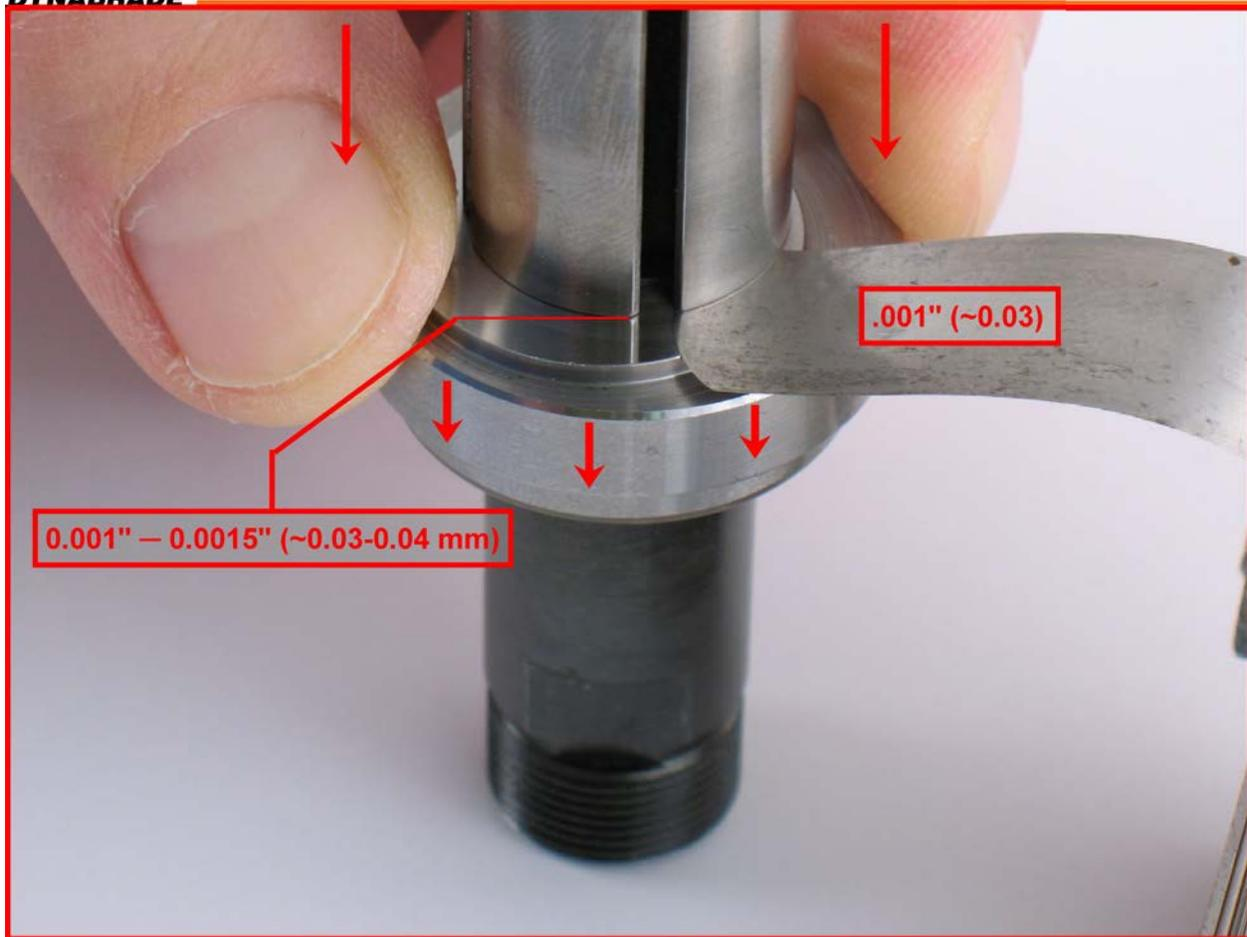
3. Install the **51922** Front Bearing Plate and bearing onto the rotor.
