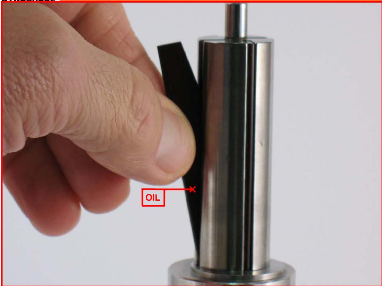
5. Apply the **95842** Dynabrade Air Lube or equivalent to the **51926** Vanes and install them into the rotor.
