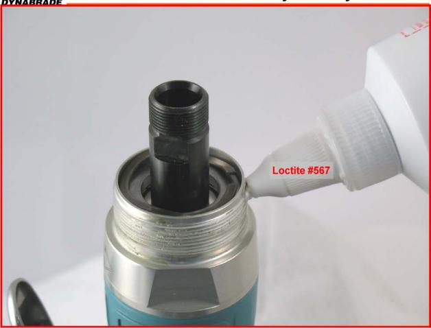
Apply a small amount of Loctite #567 to housing thread.
