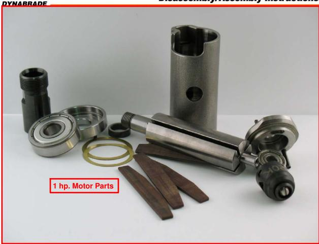
**8.** Remove the **51927** Spacer from the rotor. **Motor Disassembly Completed.**
