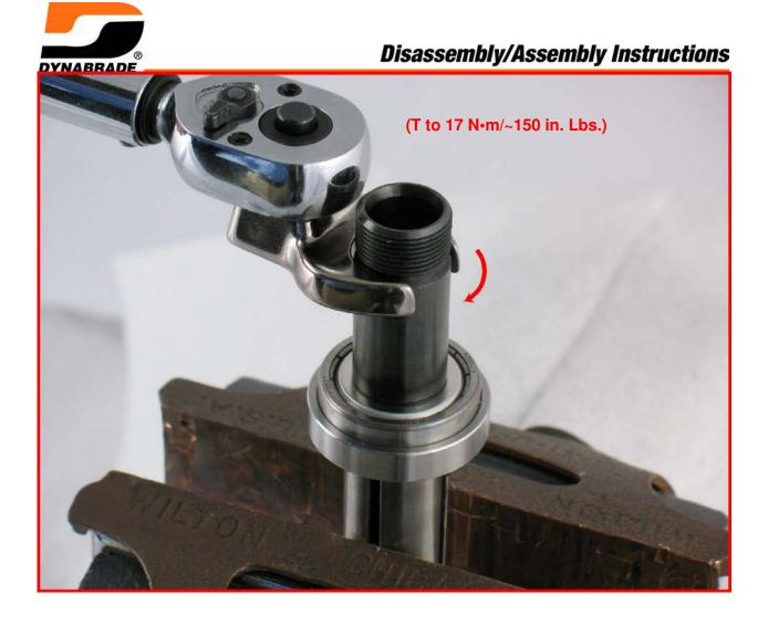
Use a 14 mm crowfoot and torque wrench to fasten the 50011 Collet Body onto the rotor. (T to 17 N•m/~150 in. Lbs.)
