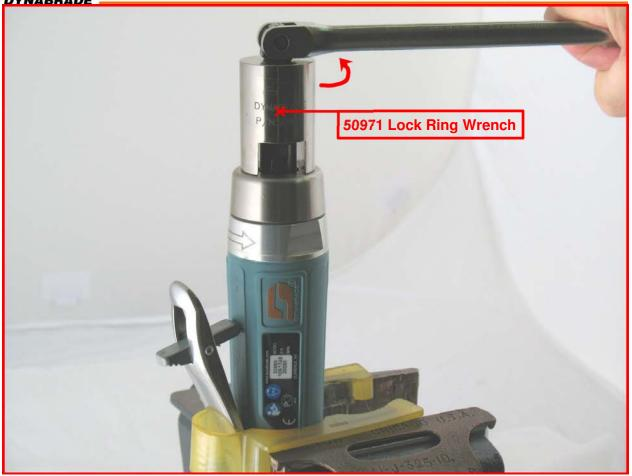
Use the 50971 Lock Ring Wrench or an adjustable pin wrench to remove the Housing Cover: 51947, 51962, 51972. Turn counterclockwise.
