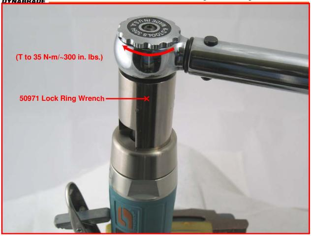
• Use the **50971** Lock Ring Wrench and torque wrench to install housing cover. (**T** to 35 N•m/~300 in. lbs.)
