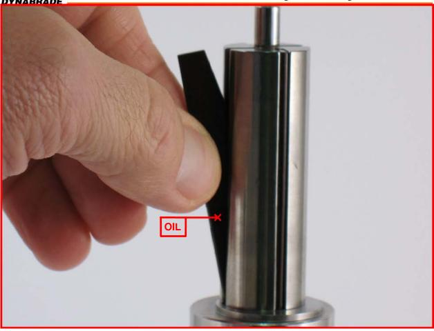
**5.** Apply the **95842** Dynabrade Air Lube or equivalent to the **51926** Vanes and install them into the rotor.
