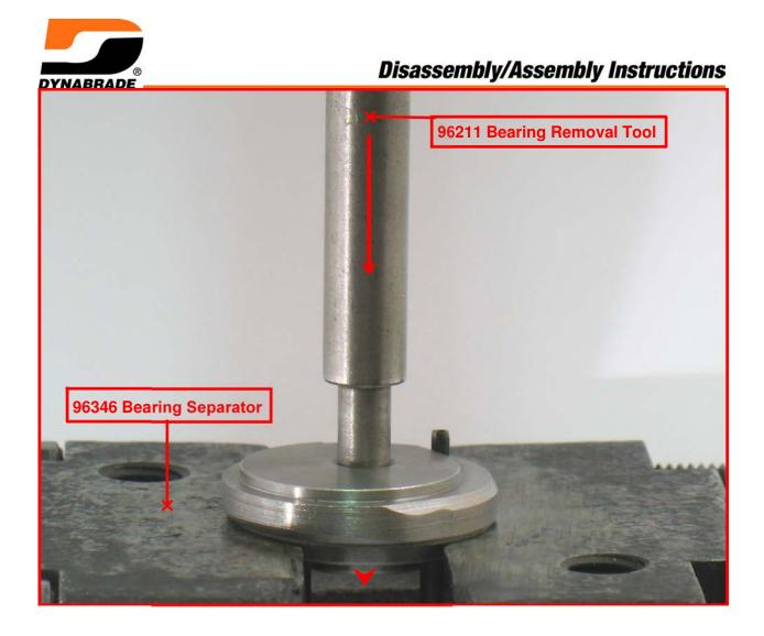
**5.** Use the **96346** Bearing Separator (2"), the arbor press and the **96211** Bearing Removal Tool to remove the **02057** Bearing from the rear bearing plate.
