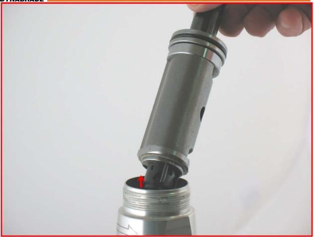
**2.** Pull-up on the work spindle to remove the motor with the **96498** Wave Spring, and the **53620** Motor Adapter from the housing.
