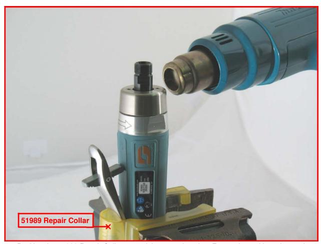
1. Position the **51989** Repair Collar around the motor housing. Fasten the tool in a vise so that the work spindle is pointing up. Use a HEAT GUN to warm the Housing Cover: **51947**, **51962**, **51972** and soften the thread adhesive.
