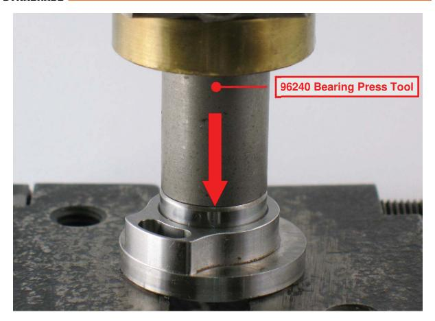
5. Use the *RAISED OUTSIDE DIAMETER* of the 96240 Bearing Press Tool and arbor press to install 02649 Bearing. **Notice:** Press bearing into plate all the way.
