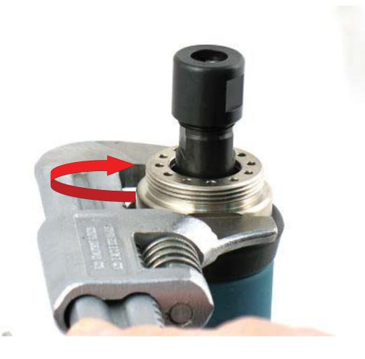
**3.** Use an adjustable wrench to remove **51870** Lock Ring. Turn counterclockwise.
