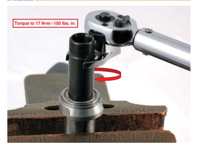
3. Use a 14 mm crowfoot and torque wrench to tighten the **50008** Collet Body. (Torque to 17 N•m/~150 lbs. in.)
