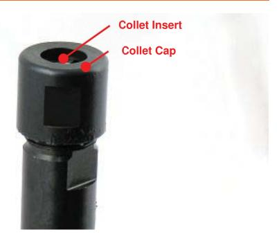
10. Install collet insert and cap to collet body.
