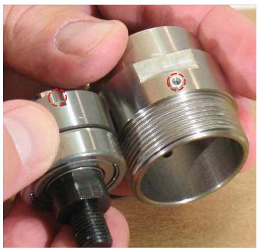
5. Install **54468** Ring Gear so that openings line-up with the lubricant and set screw holes in housing.
