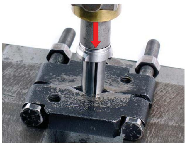
2. Use arbor press and **RAISED INSIDE DIAMETER** of the **96240** Bearing Press Tool to install **02649** Bearing with bearing plate onto rotor.
