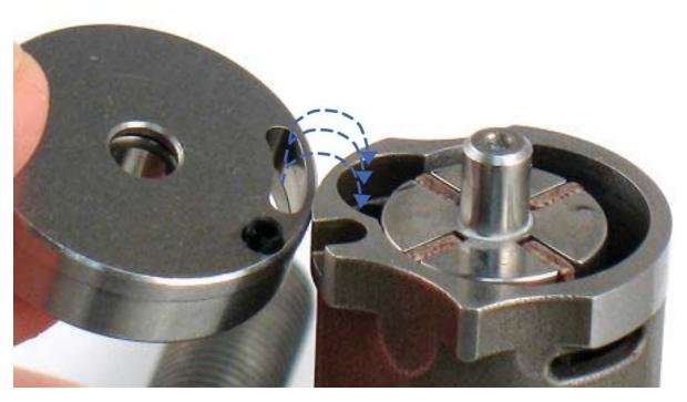
5. Install 01476 Cylinder and 02673 Rear Plate so that air inlet openings line-up.
