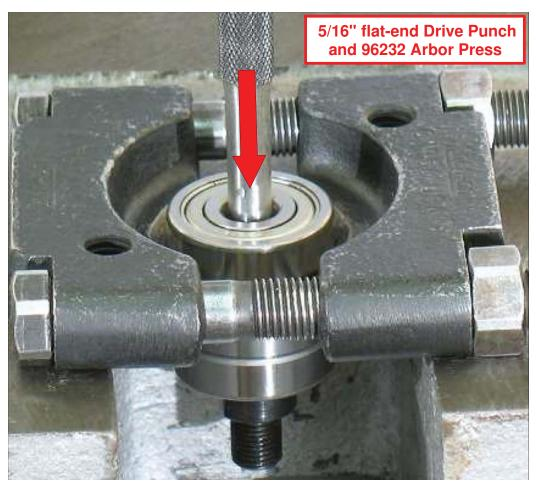
**4.** Use a 5/16" flat-end drive punch as a press tool and **96232** Arbor Press to push the planetary carrier out of the **54552** Bearing.
