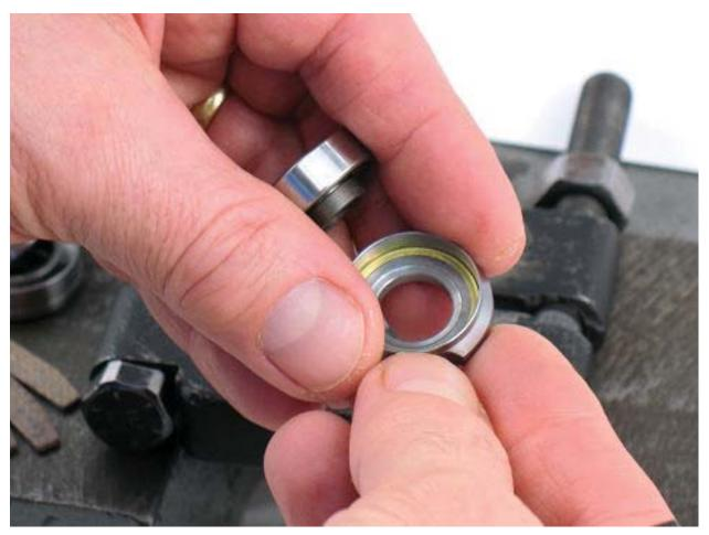
6. Remove 02649 Bearing, front plate, shims and 01479 Spacer.
