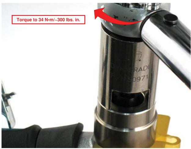
Use 50971 Lock Ring Tool and torque wrench to fasten exhaust cover. (Torque to 34 N•m/~300 lbs. in.)
