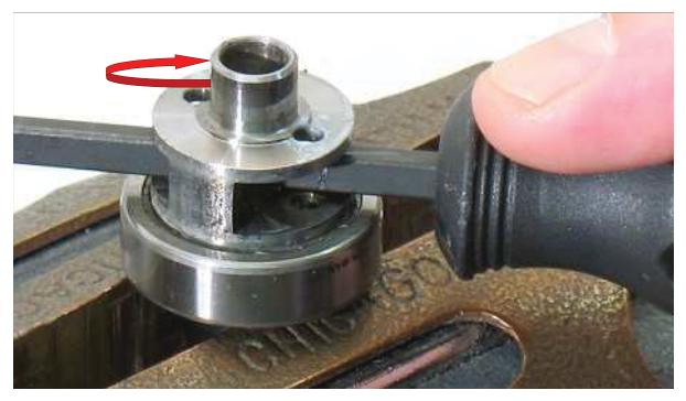
6. With planetary carrier pointing up, carefully fasten **40358** Adapter in vise with aluminum or bronze jaws. Insert a screwdriver through carrier and turn counterclockwise to remove adapter.
