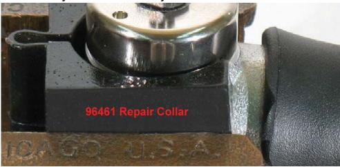
1. Use 96461 Repair Collar to hold housing in a vise with 40358 Adapter pointing up.
