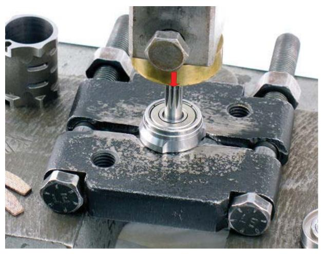
5. With pinion gear pointing up, use arbor press to push rotor out of **02649** Bearing.
