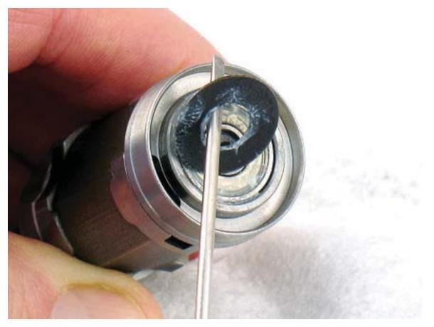
2. Remove 02679 Shield from 02696 Bearing.
