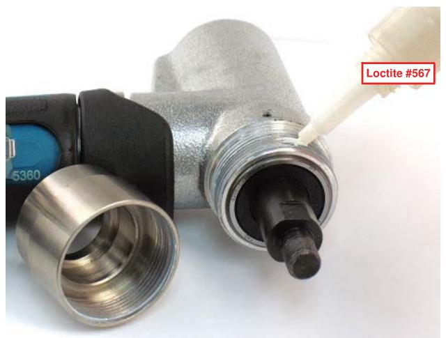
8. Apply a small amount of Loctite #567 to threads of housing.
