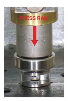
1. Use the **RAISED INSIDE DIAMETER** of the **96239** Bearing Press Tool and the arbor press to install the **54552** Bearing onto the front of the planetary carrier.
