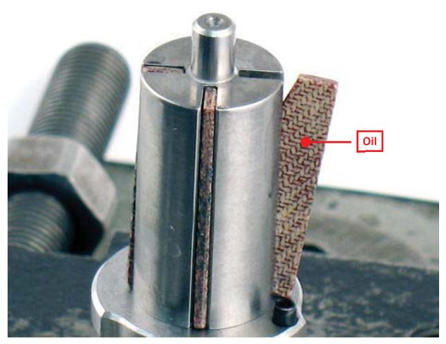
4. Oil vanes with 95842 Dynabrade Air Lube 10W/NR or equivalent, and install.
