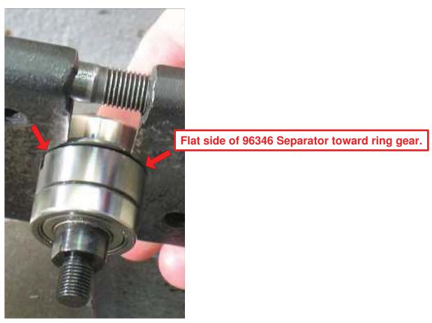
**3.** Fasten **96346** Bearing Separator between bearing and ring gear. Face flat side of separator toward ring gear and bevel side toward bearing.
