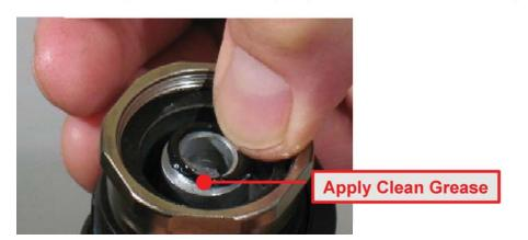
4. Apply a small amount of clean grease to **95523** O-Ring and install it onto the throttle body.
