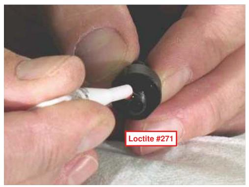
2. Apply a small amount of Loctite #271 (or equivalent) to the adapter thread.
