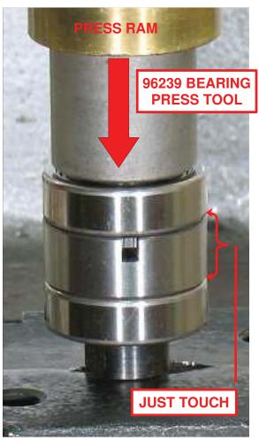
Use *RAISED INSIDE DIAMETER* of 96239 Bearing Press Tool and the arbor press to install 54552 Bearing onto planetary carrier.
