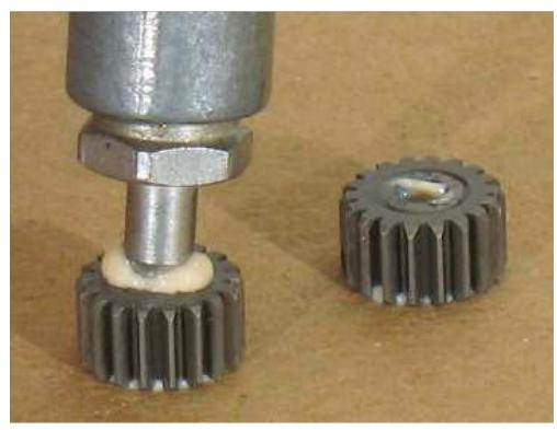
4. Apply **95542** Grease (or equivalent) to the needle bearings in the planet gears. Install gears and **54472** Shafts into carrier.
