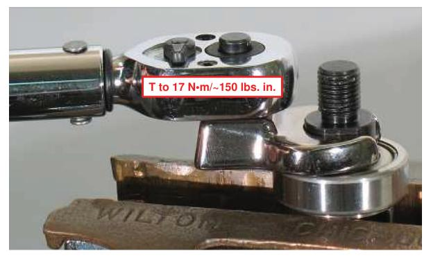
3. Carefully hold planetary carrier in vise with aluminum or bronze jaws and install the adapter onto carrier. (T to 17 N $\cdot$ m/~150 lbs. in.)
