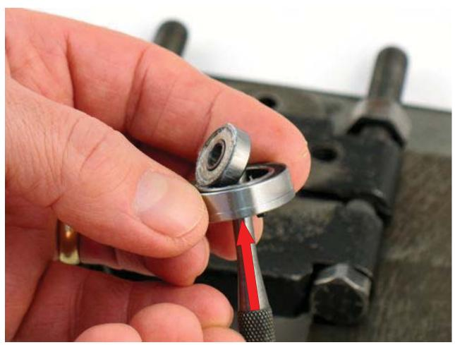
4. By hand, use Ø 3/16" or ~4 mm flat-end drive punch to push 02696 Bearing (slip-fit) out of 02673 Rear Plate.
