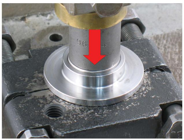
10 Use the *Raised Outside Diameter* of the 96244 Bearing Press Tool to install 01206 Bearing.
