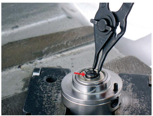
12. Install 95626 Retaining Ring into groove on shaft.
