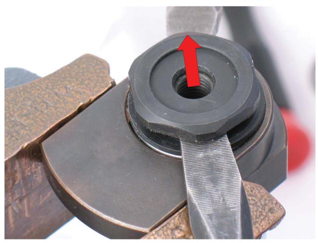
**9.** To break adhesive bond, use two large slot-blade screwdrivers to pry out balancer shaft and bearing. **Notice:** If necessary, use a HEAT GUN to warm counterweight and soften adhesive.
