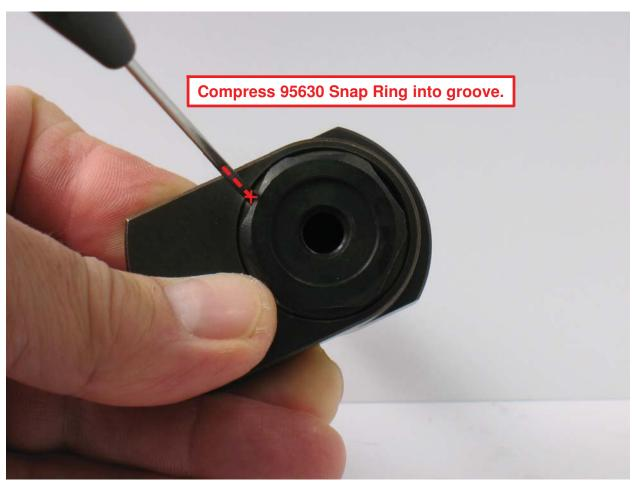
5. Use a small flat-bladed screwdriver to compress **95630** Snap Ring into groove.
