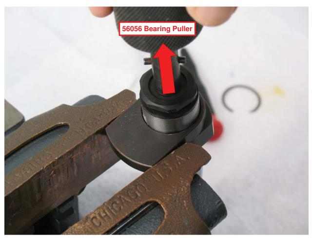
10. Use 56056 Bearing Puller to remove balancer shaft and bearing.
