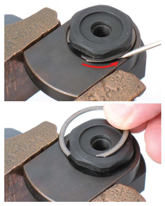
8. (continued) Slide screwdriver around counterweight to release snap ring.
