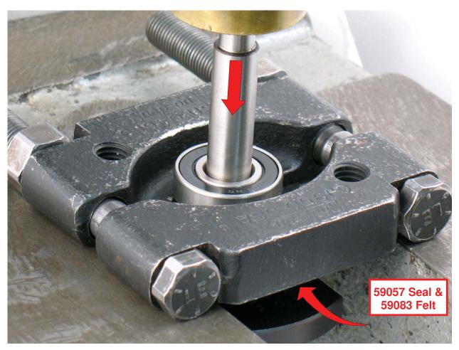
6. Use bearing separator and arbor press to remove **02695** Bearing, **59057** Seal and **59083** Felt Washer.
