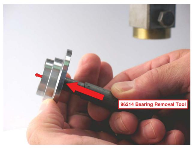
7. By hand, use 96214 Bearing Removal Tool to remove 01206 Bearing from 54629 Rear Plate.
