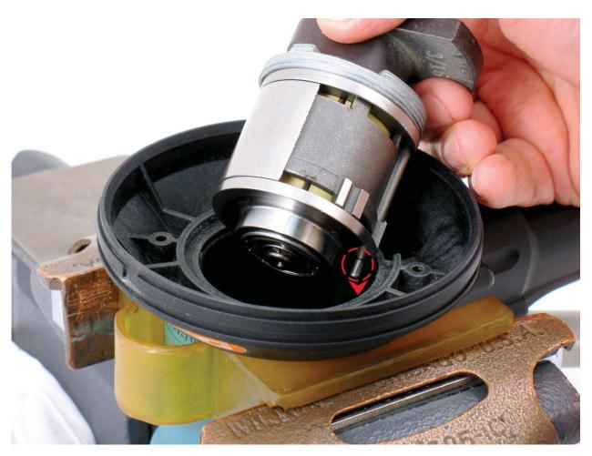
**13.** Sight line-up pin with the hole on inside of housing and install motor.
