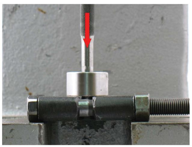
Use 5/16" or 8 mm diameter flat-end drive punch to push balancer shaft from 56052 Bearing.
