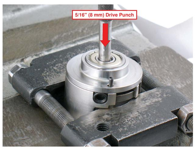
4. Use arbor press and Ø 5/16" or 8 mm flat-end drive punch to push shaft out of **01206** Bearing.
