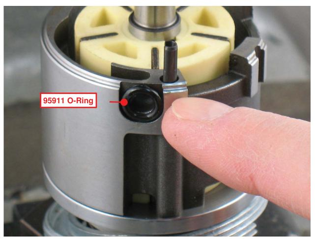
9. Apply clean grease or viscous oil to 95911 O-Ring and install in cylinder.
