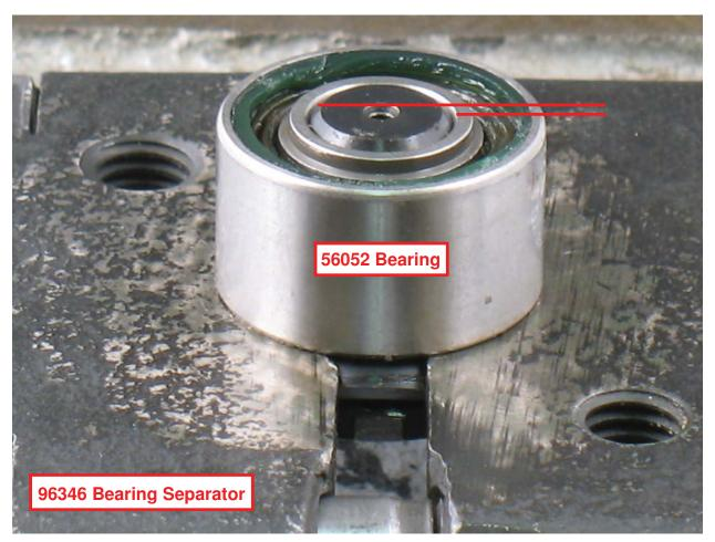
11. Fasten bearing separator between **56052** Bearing and hex end of **57069** Balancer Shaft.
