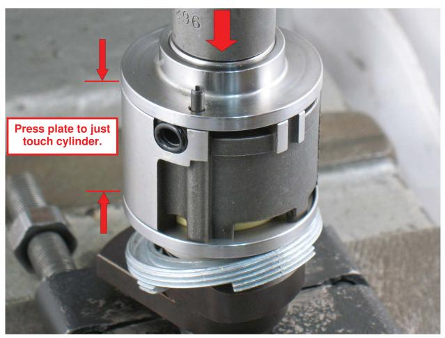
11. Use *Raised Inside Diameter* of the 96244 Bearing Press Tool to install bearing and plate onto the motor shaft balancer. Notice: Carefully press bearing and plate down until it just touches the cylinder. This will produce a close fit between the bearing plates and cylinder.
