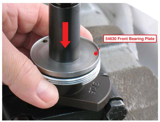
7. Use the larger end of **57091** Bearing Press Tool to install the **54630** Front Bearing Plate. **Notice:** Carefully guide lock ring and **59057** Seal to fit properly with plate.
