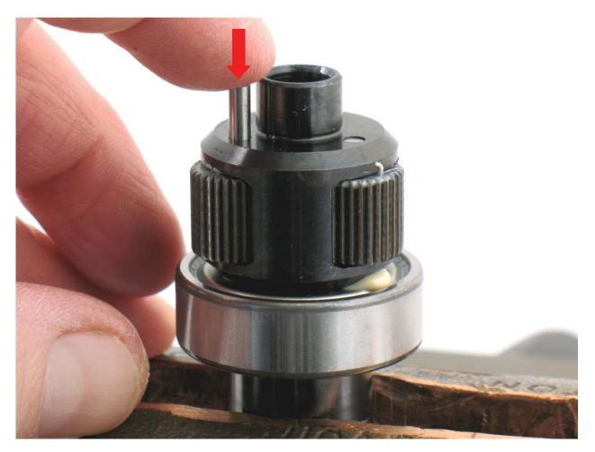
8. Install gears and 53182 Shafts into carrier.
