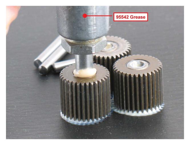
7. Apply 95542 Grease or equivalent to gears and bearings.
