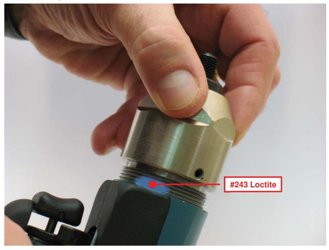
**1.** Apply #243 Loctite or equivalent to threads on gear housing.
