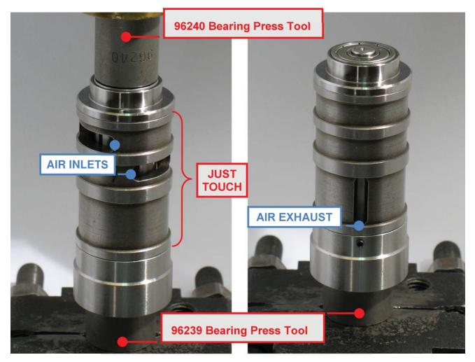
5. Use *RAISED INSIDE DIAMETER* of 96239 Bearing Press Tool to support 02651 Bearing. Use *RAISED INSIDE DIAMETER* of 96240 Bearing Press Tool and arbor press to install 02649 Bearing. Notice: Press bearing and plate down until it just touches the cylinder. This will create a close fit between the cylinder and plates.
