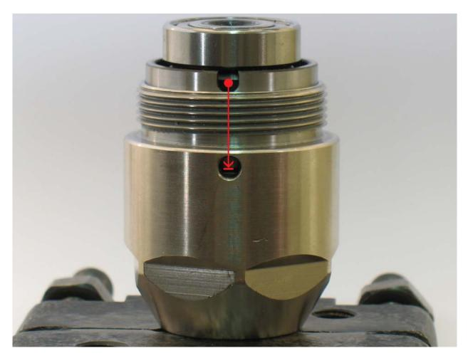
11. Install gear assembly in gear housing.
