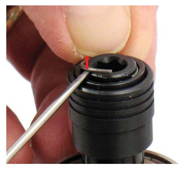
4. To disassemble "Quick Chuck", fasten carrier with spindle pointing up in vise with aluminum or bronze jaws. Use a small screwdriver or pick to remove **96592** Snap Ring.
