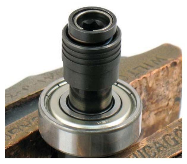
4. Install **53357** Washer and **96592** Snap Ring onto carrier spindle.
