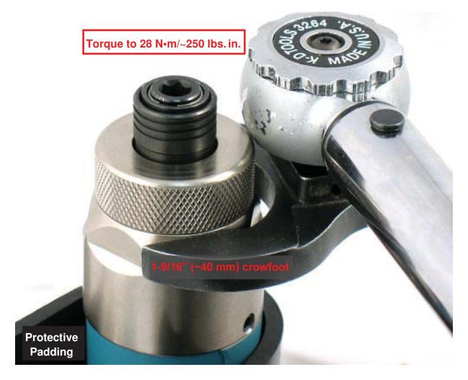
**2.** Use protective padding around housing and fasten "Driver" in vise with spindle pointing up.
