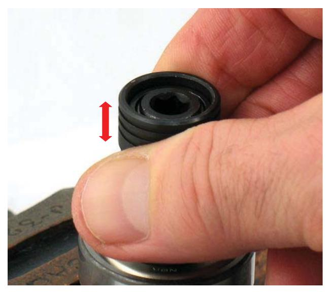
6. Pull up on **53356** Sleeve to check operation.
