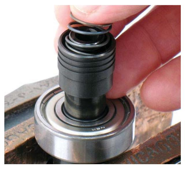
3. Install 53356 Sleeve and 53359 Spring onto carrier spindle.
