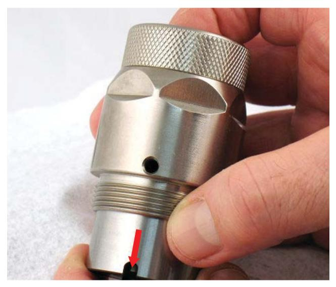
2. By hand, push spindle with gear assembly out of housing.
