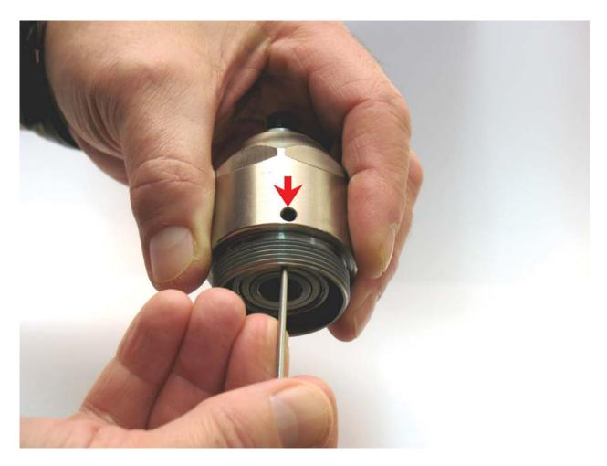
**12.** Use a small screwdriver to rotate and line-up ring gear openings with openings in gear housing.
