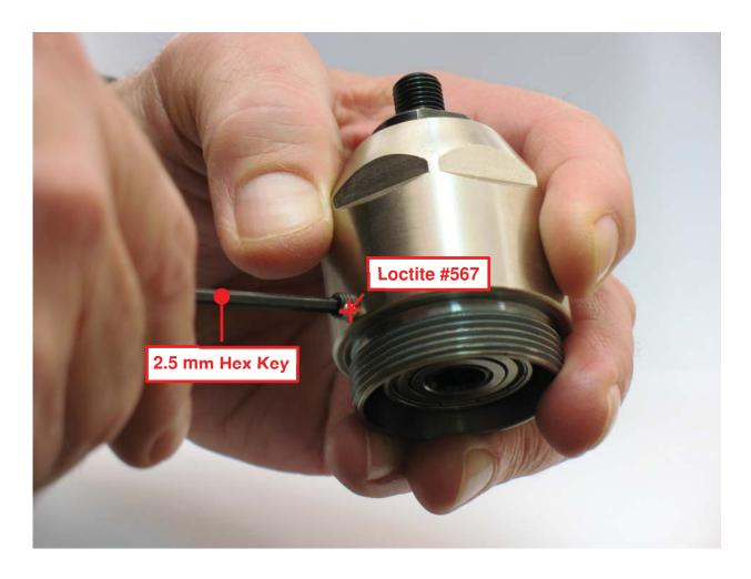
**13.** Apply a small amount of #567 Loctite to thread of **96467** Set Screw. Use a 2.5 mm hex key to install set screw.
