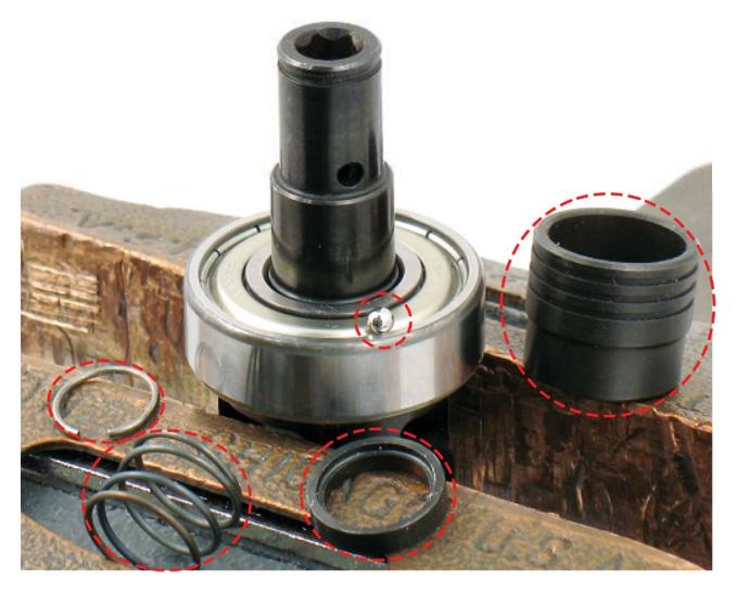
5. Remove all "Quick Chuck" components: 96592 Snap Ring, 53357 Washer, 53359 Spring, 53356 Sleeve, and 53358 Ball.
