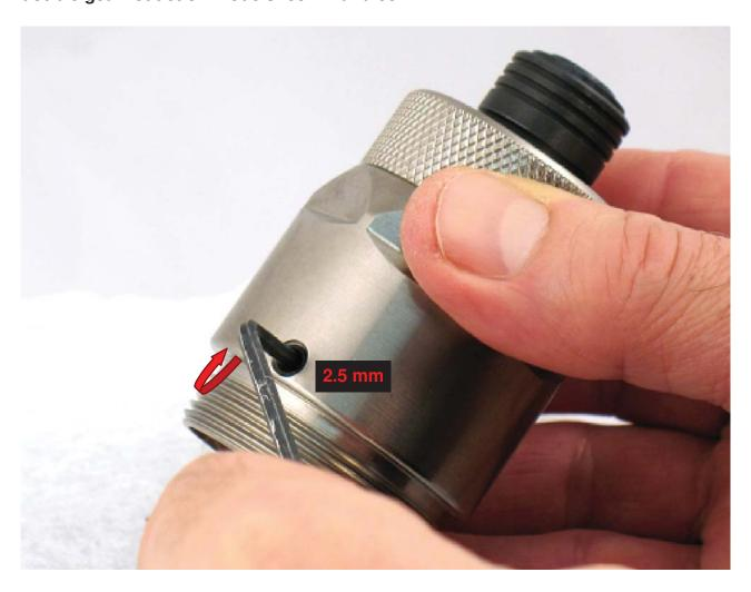
1. Use a 2.5 mm hex key to remove **96467** Set Screw. Turn counterclockwise.
