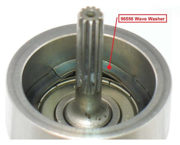
6. Install 96556 Wave Washer into 53339 Front Plate.
