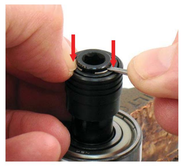
**5.** Use a small screwdriver and push down on **96592** Snap Ring and **53357** Washer to fasten snap ring into groove in spindle.
