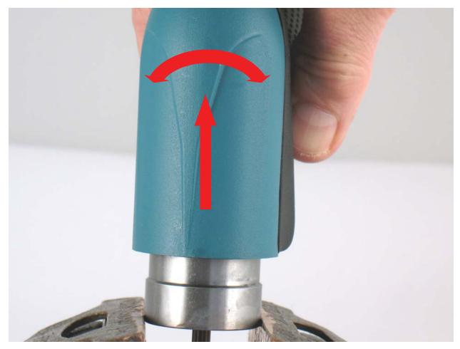
3. Pull up and wiggle housing to release motor. Remove motor from housing.
