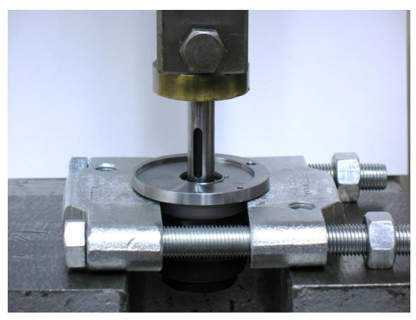
6. Use bearing separator and arbor press to remove the front bearing plate and seal.
