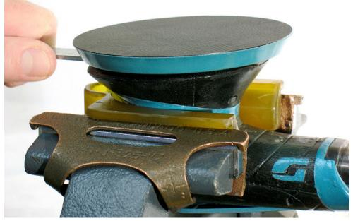
To remove sanding pad, turn counterclockwise.
