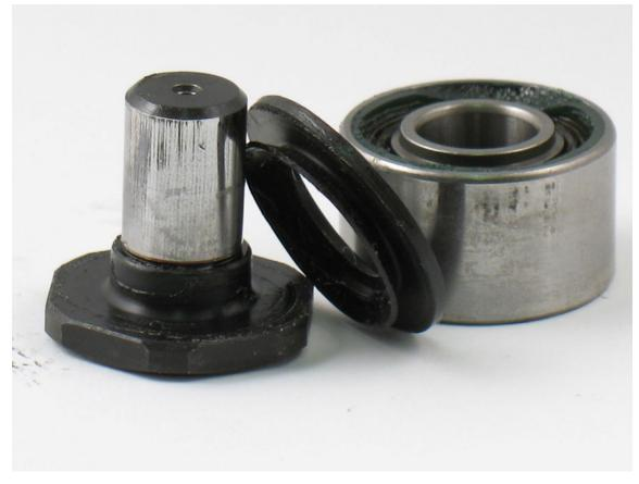
Balancer shaft and bearing disassembly completed.
