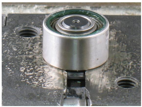
4. Fasten bearing separator between **56052** Bearing and hex end of balancer shaft.
