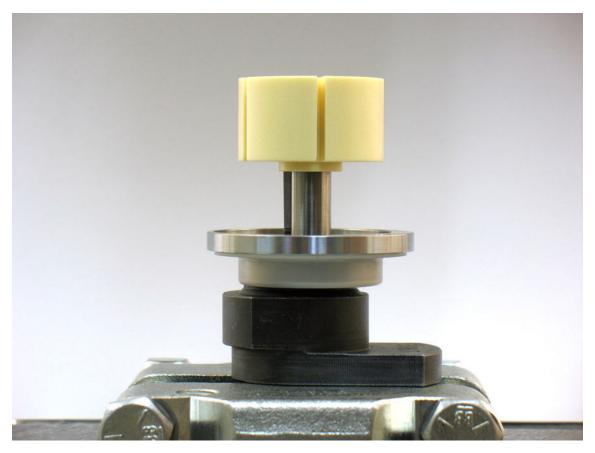
5. Remove vanes, rotor and key.
