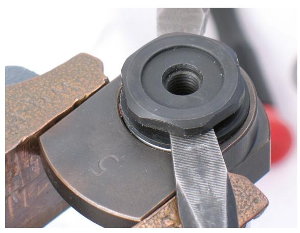
2. To break adhesive bond, use two, large slot-blade screwdrivers to pry out balancer shaft and bearing. **Notice:** If necessary, use a HEAT GUN to warm counterweight to soften adhesive.
