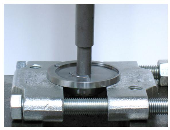
4. Use *96214 Bearing Removal Tool* to remove **58368** Bearing from **59332** Rear Bearing Plate.
