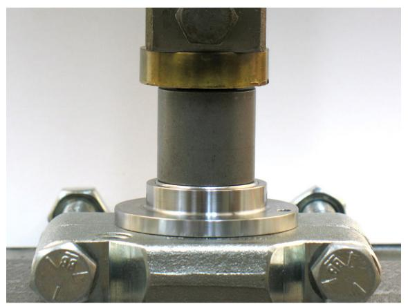
9. Use **RAISED OUTSIDE DIAMETER** of *96239 Bearing Press Tool* and arbor press to install **58368** Bearing into **59332** Rear Bearing Plate.
