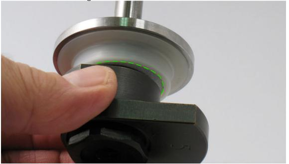
4. Carefully fit plate to the bearing, felt washer and front bearing seal. Notice: The felt washer should be completely retained in the front bearing seal.
