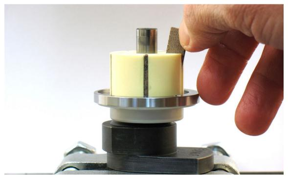
6. Apply **95842** Dynabrade Air Lube 10W/NR or equivalent to vanes and install.
