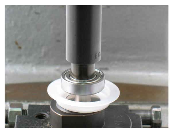
2. Use small diameter of *57091 Bearing Press Tool* and arbor press to install **58368** Bearing onto shaft balancer.
