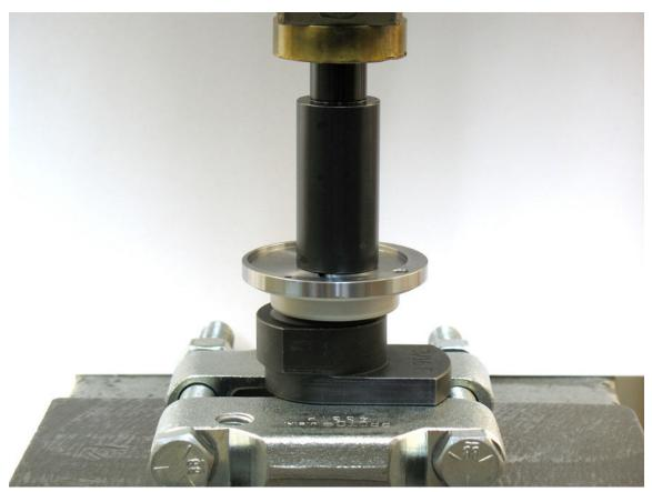
3. Use large diameter end of *57091 Bearing Press Tool*, and arbor press to install **59333** Front Bearing Plate.
