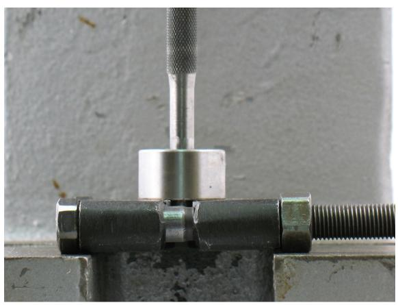
6. Use a 5/16" or 8 mm diameter flat-end drive punch as a press tool to push balancer shaft out of **56052** Bearing.
