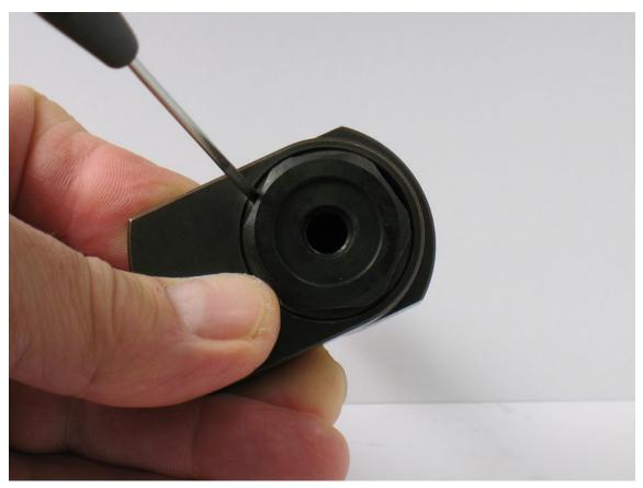
5. Use a thin slot-blade screwdriver to compress and install **95630** Snap Ring into groove of shaft balancer.
