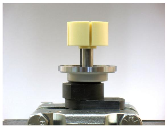
5. Install **56047** Key and rotor onto shaft balancer.
