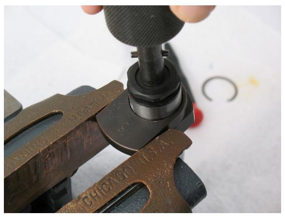
3. Use *56056 Bearing Puller* to remove balancer shaft and **56052** Bearing.
