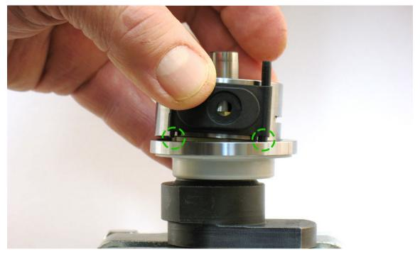
8. Install **59134** Cylinder Sleeve and **59133** Cylinder Sleeve Adapter so that short pins fit into front bearing plate.
