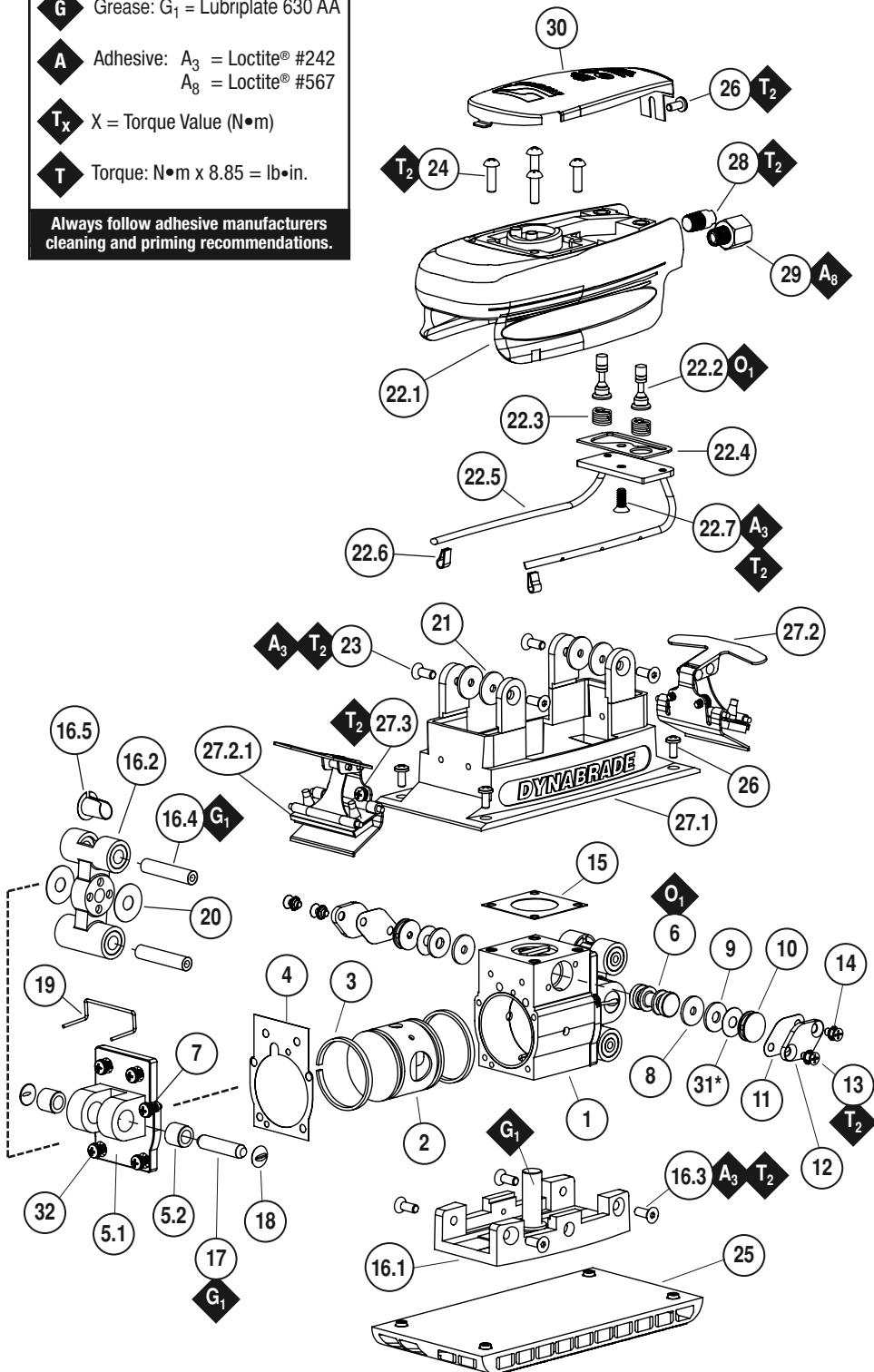
\*ITEM 31 ONLY USED TO SHORTEN THE STROKE OF THE PISTON, WHEN PISTON HITS END PLATES
