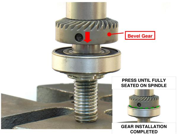
2. Use press to install bevel gear onto spindle.
