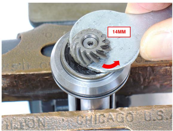
9. Use **95262** Wrench (14mm) to remove pinion gear. Turn counterclockwise.
