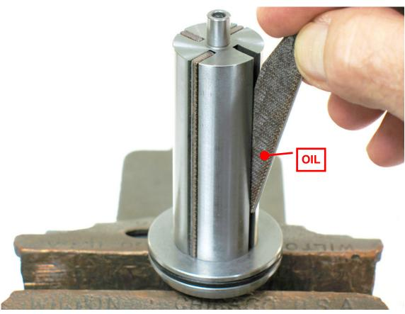
6. Apply **95842** Dynabrade Air Lube 10W/NR or equivalent to **54904** Vanes and install.
