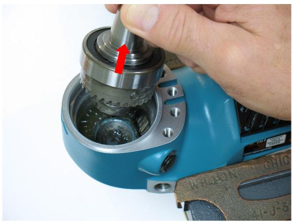
2. Remove work spindle assembly from housing.
