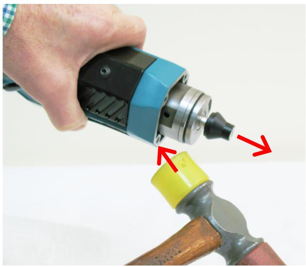
4. Use soft-faced hammer to knock motor assembly loose from housing and remove.
