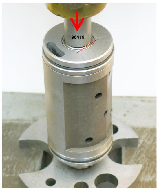
9. Use the *RAISED INSIDE DIAMETER* of 96419 Bearing Press Tool, and the arbor press to install rear bearing.
