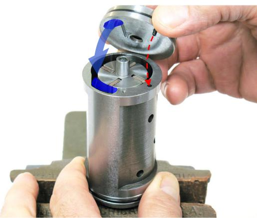
7. Install **54905** Cylinder and rear end plate so that air inlet openings line up.
