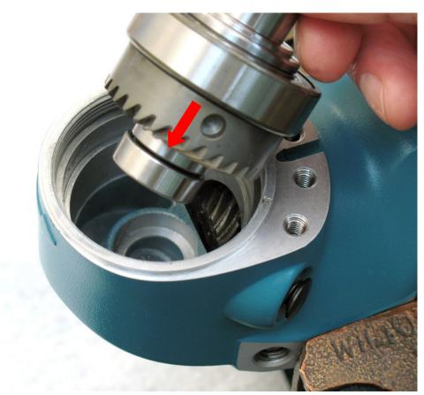
4. Fasten housing in vise (bronze or aluminum jaws). Install spindle assembly in housing.
