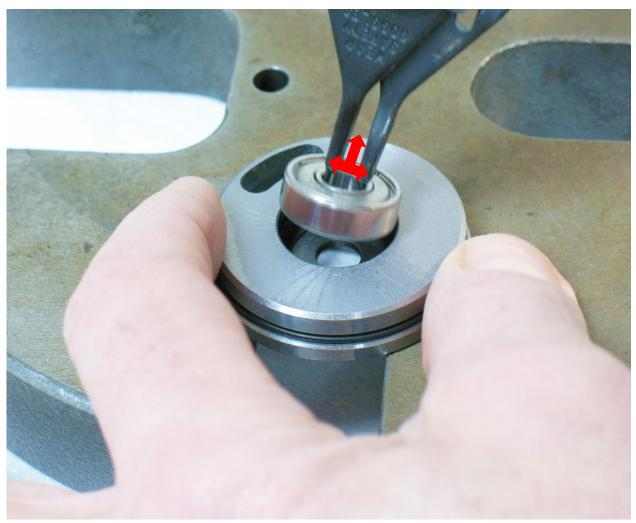
7. Use external ring pliers to remove **54907** Bearing from **54880** Rear End Plate.
