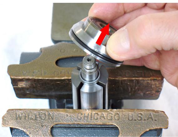
10. Remove; **54900** Bearing, **54901** Front End Plate along with shims and **54902** Spacer.
