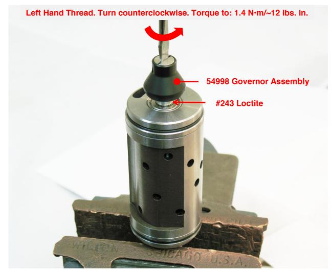
10. Carefully, fasten pinion gear in vise (bronze or aluminum jaws).
