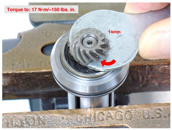
4. Use 14mm Wrench (or thin crowfoot) to fasten pinion gear. Turn clockwise.
