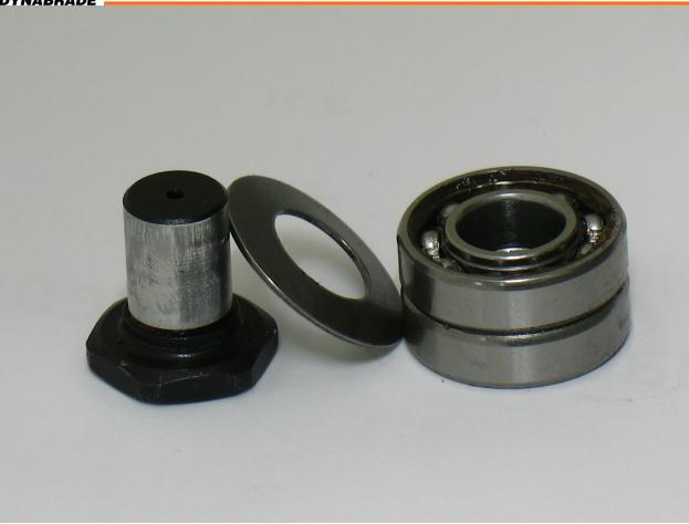
Balancer shaft and bearing disassembly completed.
