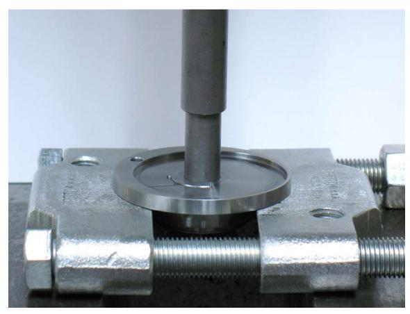
4. Use **96214 Bearing Removal Tool** to remove **01139** Bearing from **59405** Rear Bearing Plate.
