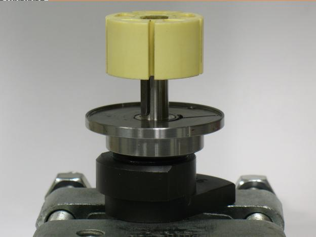
5. Remove vanes, rotor and key.
