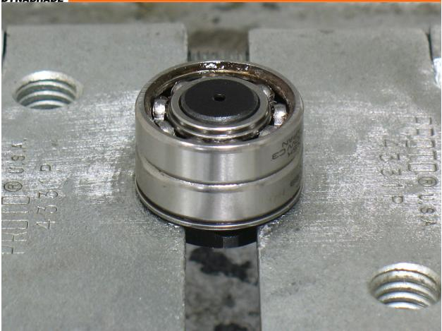
4. Fasten bearing separator between **95612** Spring (bearing shield) and hex end of balancer shaft.
