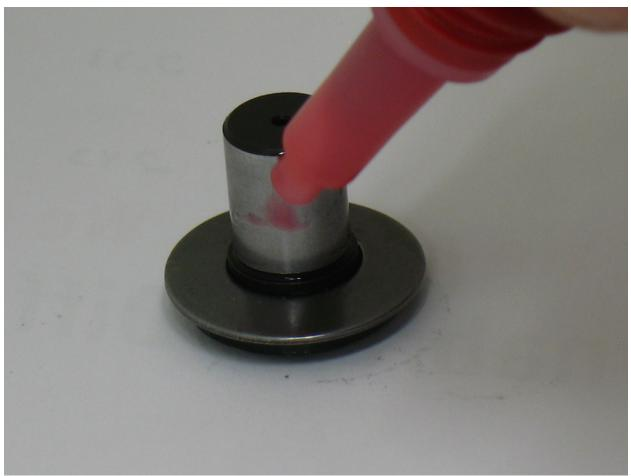
2. Apply a small amount of Loctite #271 or equivalent to outside diameter of balancer shaft.
