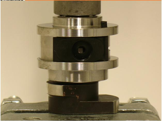
7. Use **RAISED INSIDE DIAMETER** of **96244 Bearing Press Tool** and arbor press to install bearing and plate onto shaft balancer.
