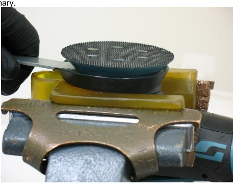
To remove sanding pad, turn counterclockwise.
