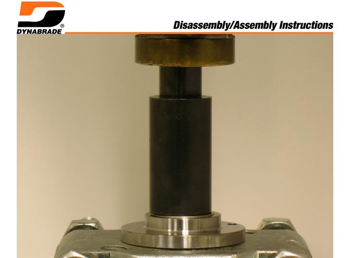
6. Use **LARGE DIAMETER END** of **57091 Bearing Press Tool** and arbor press to install **01139** Bearing into **59409** Rear Bearing Plate.
