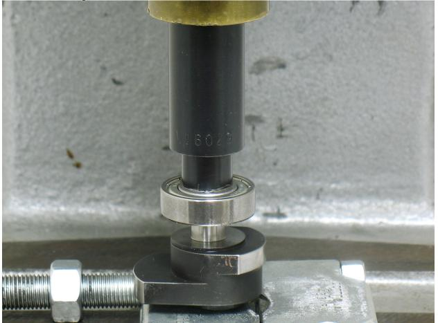
1. Use small diameter of **57091 Bearing Press Tool** and arbor press to install **58368** Bearing onto shaft balancer.
