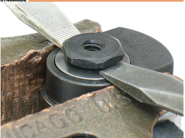
2. To break adhesive bond, use two, large slot-blade screwdrivers to pry out balancer shaft and bearing. **Notice:** If necessary, use a HEAT GUN to warm counterweight to soften adhesive.
