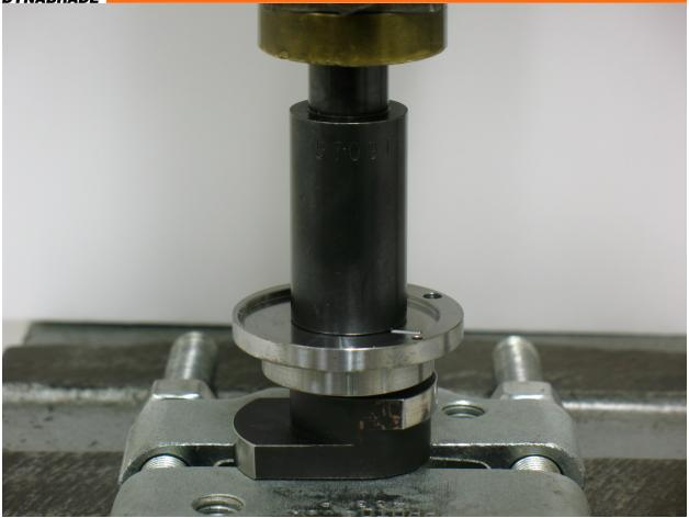
2 Use large diameter end of **57091 Bearing Press Tool**, and arbor press to install **59408** Front Bearing Plate.
