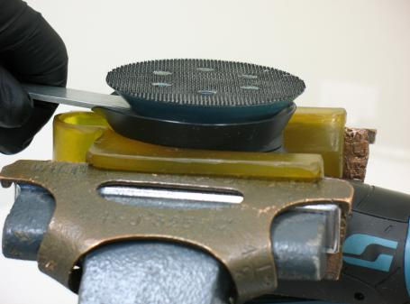
To remove sanding pad, turn counterclockwise.
