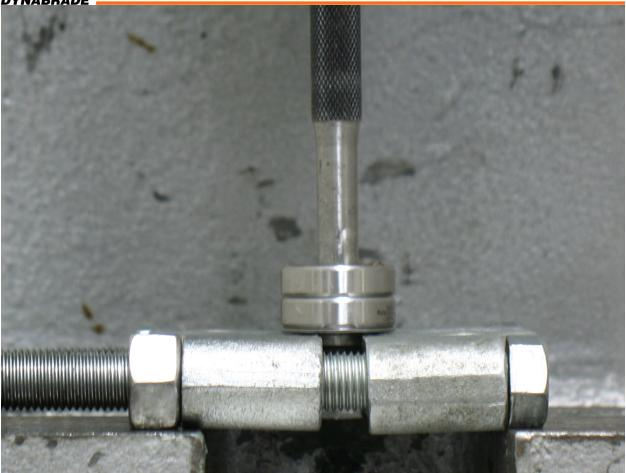
6. Use a 5/16" or 8 mm diameter flat-end drive punch as a press tool to push balancer shaft out of **59416** Bearings.
