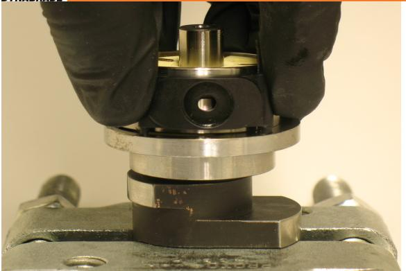
5. Install **59411** Cylinder Sleeve and **591412**Cylinder Sleeve Adapter so that short pins fit into front bearing plate.
