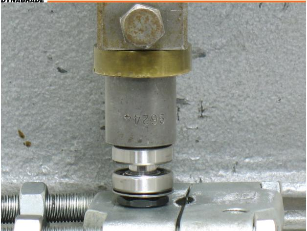
3c. Use small diameter of **96244 Bearing Press Tool** and arbor press to install second **59416** bearing with no seals, in the same manner as the first.
