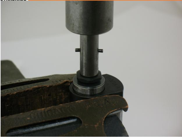
3. Use **54141 Bearing Puller** to remove balancer shaft and **59416** Bearings (2).
