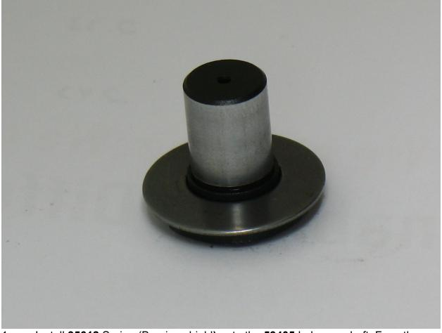
1. Install **95612** Spring (Bearing shield) onto the **59405** balancer shaft. Face the convex side of the spring (bearing shield) toward the hex end of the balancer shaft
