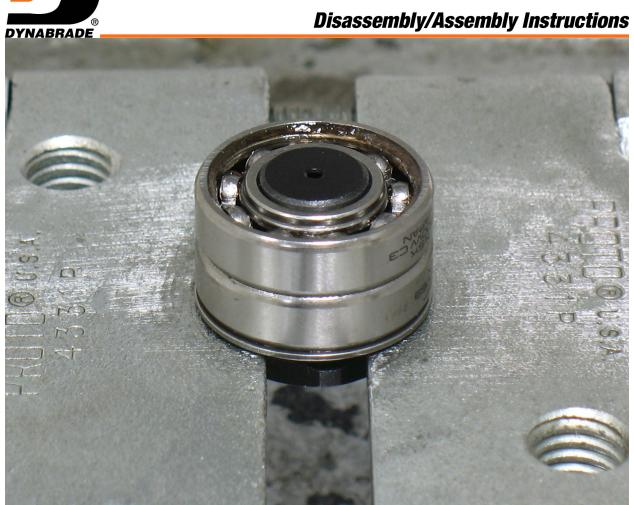
4. Fasten bearing separator between **95612** Spring (Bearing Shield) and hex end of balancer shaft.
