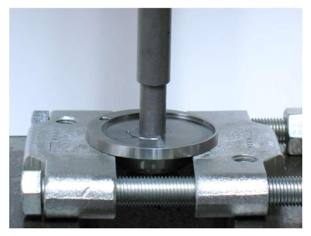
4. Use **96214 Bearing Removal Tool** to remove **01139** Bearing from **59405** Rear Bearing Plate.
