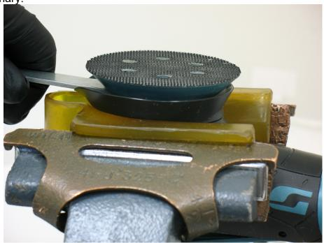
To remove sanding pad, turn counterclockwise.
