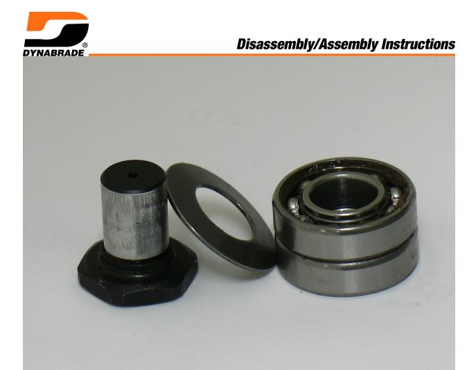
Balancer shaft and bearing disassembly completed.
