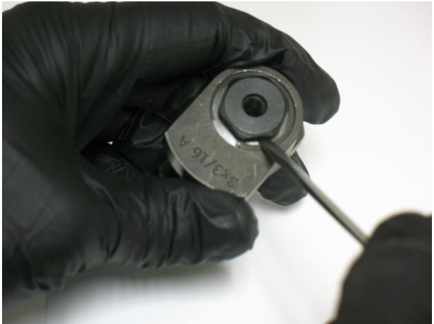
5. Use a thin slot-blade screwdriver to compress and install **95613** Snap Ring into groove of shaft balancer.
