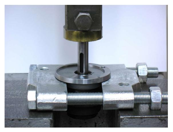
6. Use bearing separator and arbor press to remove the front bearing plate.
