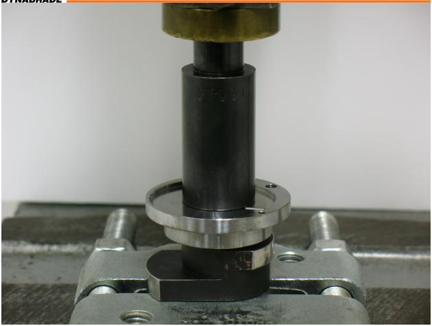
Use large diameter end of **57091 Bearing Press Tool**, and arbor press to install **59408** Front Bearing Plate.
