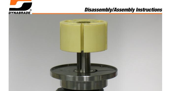
5. Remove vanes, rotor and key.
