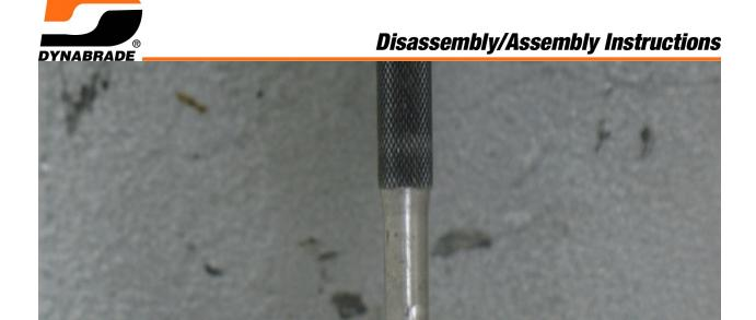
6. Use a 5/16" or 8 mm diameter flat-end drive punch as a press tool to push balancer shaft out of **59416** Bearings.
