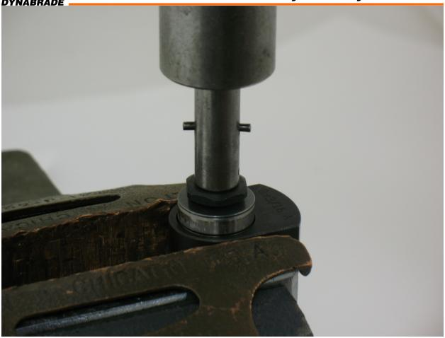
3. Use 54141 Bearing Puller to remove balancer shaft and 59416 Bearings (2).
