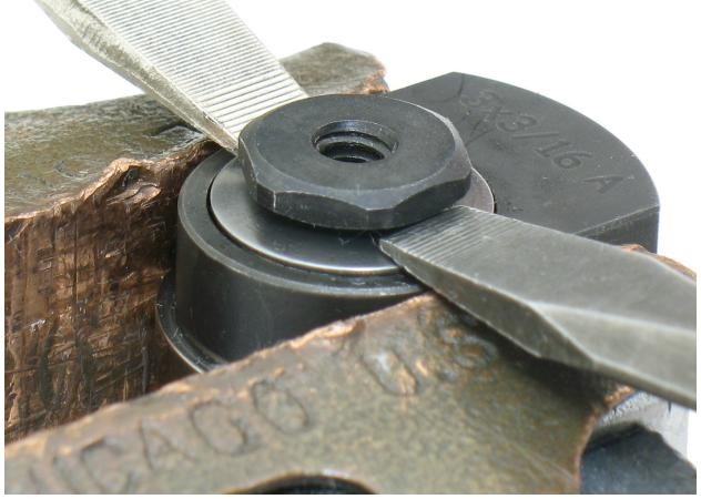
2. To break adhesive bond, use two, large slot-blade screwdrivers to pry out balancer shaft and bearing. **Notice:** If necessary, use a HEAT GUN to warm counterweight to soften adhesive.
