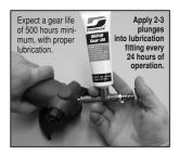
Lubricate wick system through the angle gear oil fitting with 2-3 plunges for every 24 hours of use, to achieve maximum gear life. Prime pump to insure good oil flow.
