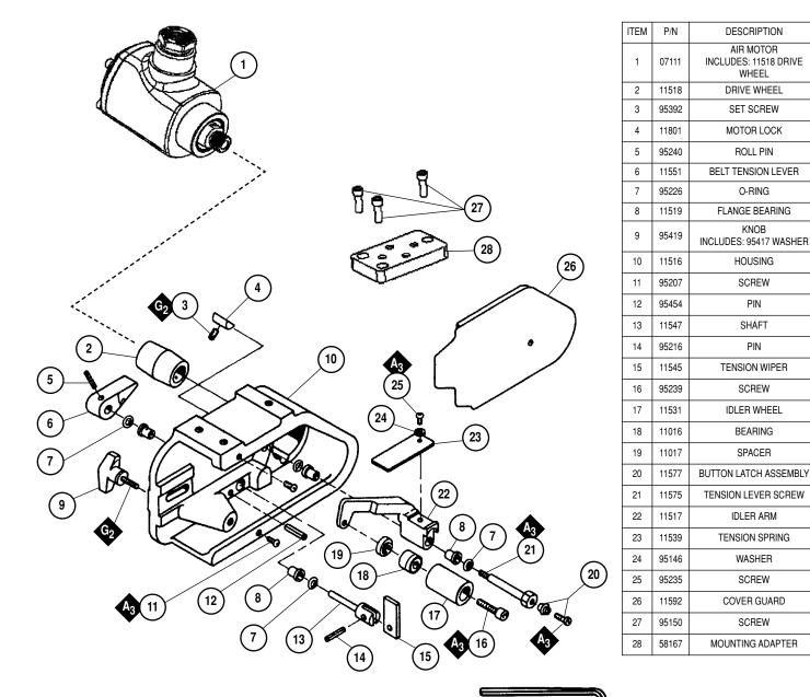
Wrench Fits **95392** Screw for adjusting motor position.
