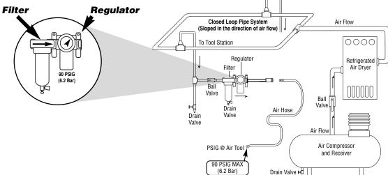
This tool should use filtered and regulated air, but does not require lubricated air. Lubricated air is not detrimental to tool life.
