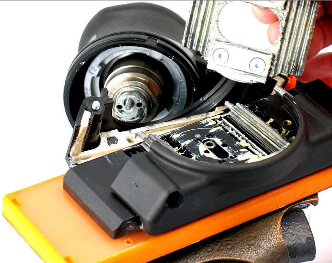
2. Separate **57427** Slider Housing halves.
