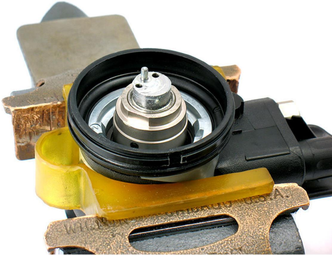
3. To add grease to the planetary gear assembly, use **57092** Collar to hold housing in vice.
