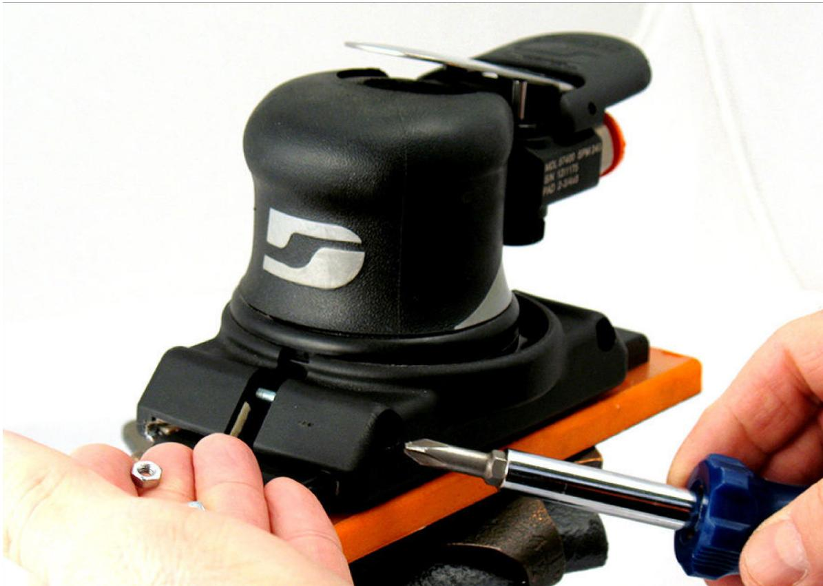
1. Remove **95642** Screws (2) and **95641** Hex Nuts with Phillips screwdriver.
