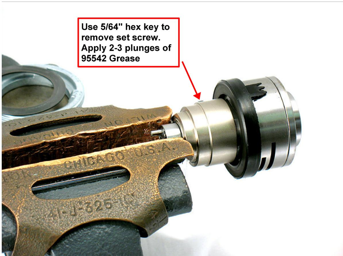
6. Use a 5/64" (2 mm) hex key to remove the **95593** Set Screw. Turn counterclockwise.
