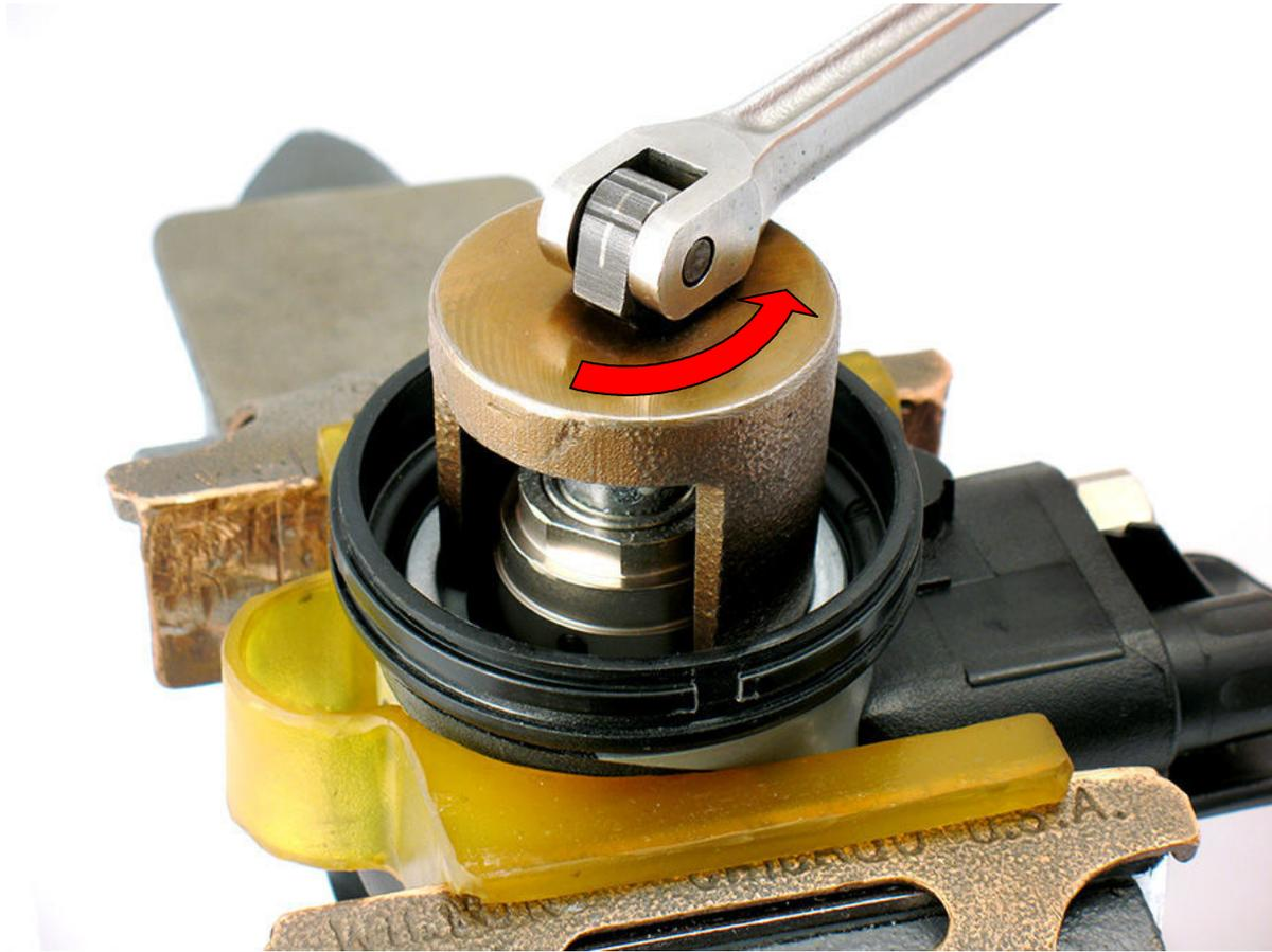
4. Use **56058** Lock Ring Wrench to remove lock ring. Turn counterclockwise.
