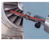
Efficiently rework turbine blades with specialized contact arm.
