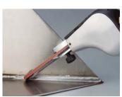
Grind welds using belts as narrow as 1/8" wide.
