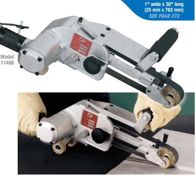
Place 11486 Dynabelter handle at 45° angle from belt housing to increase grinding pressure. Pull tool toward operator for faster material removal.
