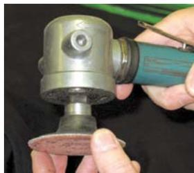
"The spindle won't turn." This usually indicates broken vanes.
