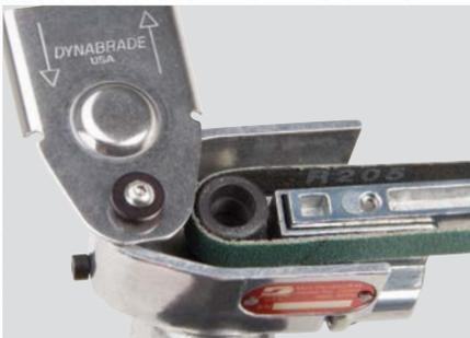
The belt housing on mini-belt tools swings open for easy abrasive changes without the need for extra tools.
