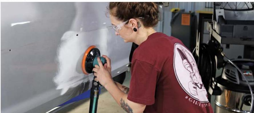
The Dynorbital-Spirit® is the lightest random orbital sander from Dynabrade and is ideal for vertical feather-edging applications where technicians are working in front of their body or at eye level with a vehicle raised on a lift. Weighing less than two pounds the Spirit sander reduces operator fatigue and relieves stress on wrists and arms. Improve shop air quality by combining with Dynabrade Mini-Raptor Vacs®.
