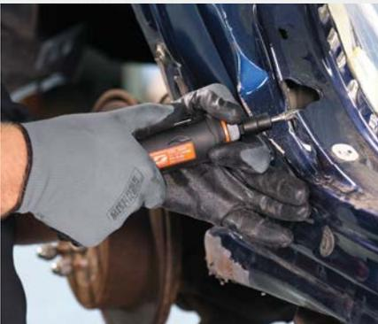
Die Grinders provide a great deal of options for technicians within the body shop. Having a 1/4" collet allows for the use of burs along with coated and non-woven abrasives in a variety of shapes and sizes.
