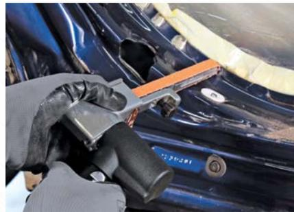
Using a belt rather than a drill bit is a quick, efficient and economical way to remove spot welded panels while leaving material to reattach the new or repaired panel.
