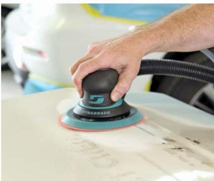
The Dynorbital® Extreme coupled with a Raptor Vac® significantly reduces dust within a garage. Airborne dust settling on painted surfaces is a major cause of rework and delays in moving vehicles through the repair process. The Extreme Sanding System provides best-in-class dust extraction contributing to an efficient repair process while also protecting technicians from potentially harmful respirable dusts.
