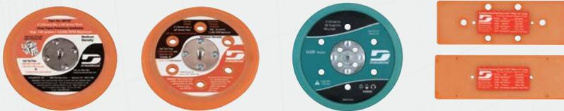
Sanding pads are more than a component that an abrasive disc or sheet attaches to; they are a critical component to creating the finest, most consistent surface finishes. Dynabrade random orbital sanding pads are weight-mated to each pad diameter, reducing vibration that leads to poor finishes and ergonomic concerns for the user. The single-piece hub design is a feature pioneered by Dynabrade that further reduces
