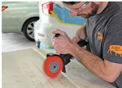
Using an eraser wheel the Dynabrade Nitro Series™ NitroZip quickly removes decals without harming the paint below, as well as removing adhesives without smearing on the painted surface.
