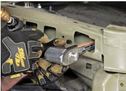
Grinding hard to reach spot welds, or even through a seized or stripped bolt is easy with Dynabrade belt tools that allow technicians to access tight areas with greater control.
