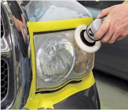
Dynabrade offers small diameter buffers for use on headlights and small areas where other buffers cannot reach or maneuver around. Pictured here is a Sander/Buffer combination tool that allows technicians to toggle between rotary and random orbital motions with the flip of a switch. Providing versatile tools that can accomplish multiple tasks is one way Dynabrade helps maximize productivity.
