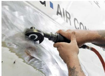
Cutting through panels is easy and accurate using Dynabrade cut-off tools. Powerful air motors drive abrasive wheels efficiently, and the variety of formats - straight, offset, right angle - allow operators greater control in their application.
