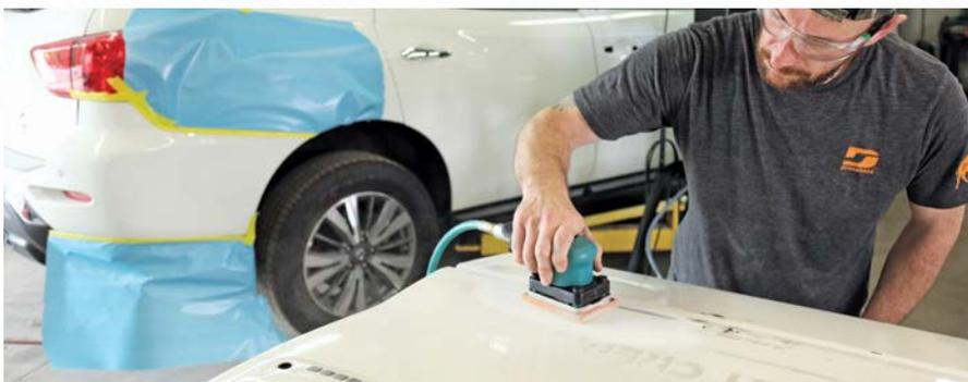
Dynabug® sanders are an ideal choice for use in feather edging applications. The square pad and delicate orbital motion allow technicians to sand in corners without undercutting. When equipped with a long-nap pad and non-woven nylon abrasives Dynabug® and Dynabug®II sanders are excellent scuffing and blending tools.
