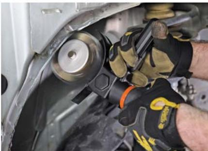
When equipped with a wire wheel the Dynabrade Nitro Series™ NitroZip removes seam sealer quickly and without clogging leaving the surface below ready for rework.
