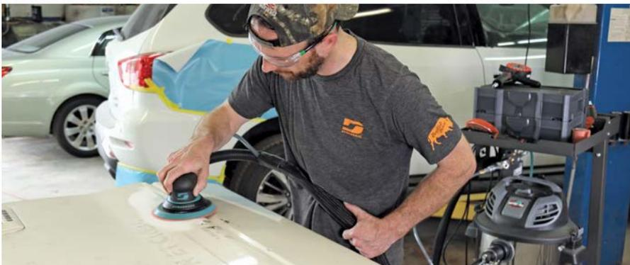
The Mini-Raptor Vac® Pro-Pack provides technicians with a complete package for all their sanding, storage and mobility needs. The single tech work station seen here is easily expandable to a two-person station by adding a Y-connector and second hose. The shelf and storage containers keep additional tools and abrasives organized and close at hand, while the small footprint keeps floor space free of clutter.
