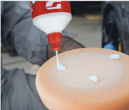
When establishing a final finish, it is important to apply compound to the surface of the pad and then blot additional compound on the area to be polished. Because of the self-diminishing abrasive technology in Dynabrade compounds it is critical to have fresh compound throughout the area to be polished, adhering to this step will ensure even and consistent results.
