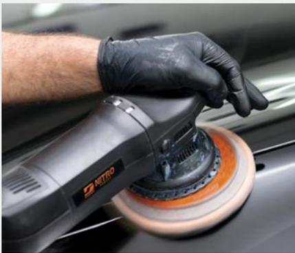
The Dynabrade finishing system consisting of buffers, pads and compounds can be seen here achieving a high-gloss, showroom finish on a dark painted front quarter panel. The buffer is easily controlled having two grip points, while the buffing pad conforms to the contours of the vehicle creating a consistent finish.
