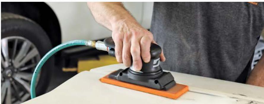
The in-line sanding motion of a Dynaline sander provides technicians with a powered option for completing traditional hand blocking applications. When used with non-woven abrasives Dynaline sanders are a great option for scuffing and surface preparation applications.
