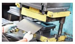
**STAMPING PLANTS APPLICATIONS:** Polishing stamping dies, breaking sharp edges, die maintenance.
