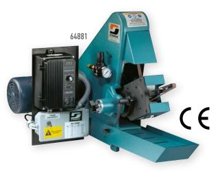
64881 - 1 hp, 230 V(AC), 1 Phase, 50Hz, 600-4,000 SFPM, for 1/4"-2" wide by 72" long belts. CE certified.
