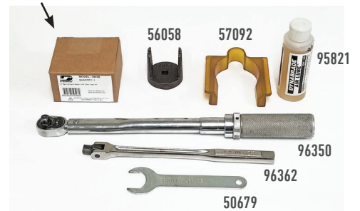
Tools needed for proper repair of orbital sanders
